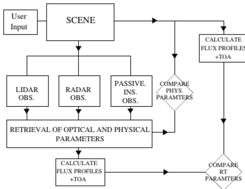
Figure 1: Schematic depiction of the ‘end-to-end’ simulation concept including the radiative closure assessment.
