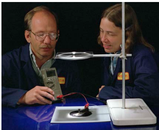
This archive photo shows NREL scientists Jerry Olson and Sarah Kurtz testing the voltage of their award-winning gallium indium phosphide/gallium arsenide solar cell, which had achieved record efficiencies, converting more than 30% of incident sunlight into electricity.
