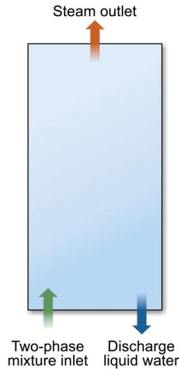
Figure 1. Diagram of a separator dryer component.
