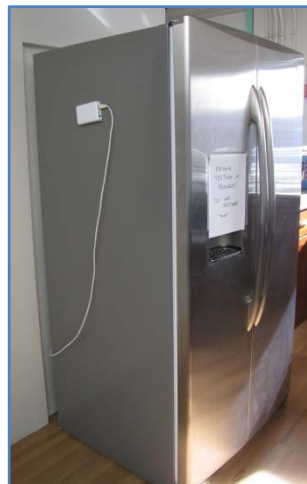
Figure 3. The smart refrigerator with the ACM connected via an Ethernet cable
