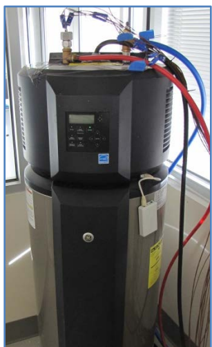
Figure 1. GE's GeoSpring hybrid HPWH (L) and Profile smart appliances (R). Each appliance can report its own energy use and respond to utility price signals via the Nucleus home energy management system.
