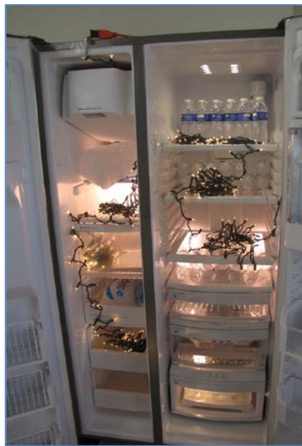
Figure 12. The inside of the refrigerator and freezer including the thermal mass (water bottles and ice) and incandescent light strings uses to simulate load
