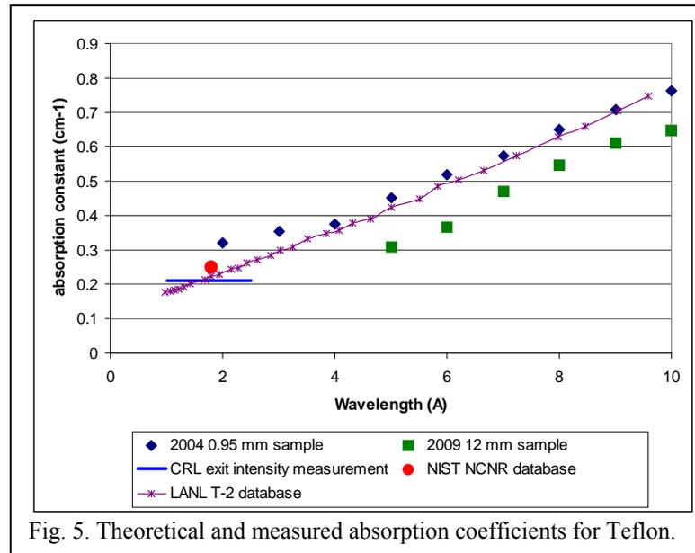
Fig. 5. Theoretical and measured absorption coefficients for Teflon.
