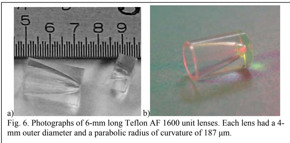
Fig. 6. Photographs of 6-mm long Teflon AF 1600 unit lenses. Each lens had a 4-mm outer diameter and a parabolic radius of curvature of 187  $\mu\text{m}$ .
