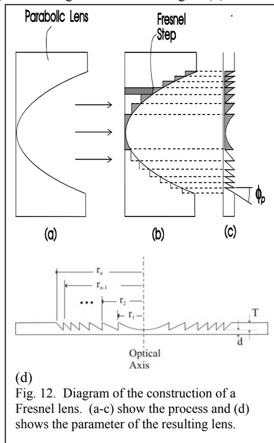
necessary manufacturing precision, alignment, etc. For the Fresnel lens, the steps are placed such that the power absorption is reduced by the factor  $e^{-a}$ , where  $a = \mu NT$ , with  $T = \frac{1}{2R}(r_n^2 - r_{n-1}^2)$  being the thickness of the unit lens,  $N$  the number of unit lenses, and  $\mu$  the power absorption constant. With this condition, the step locations,  $r_n$ , are given by
