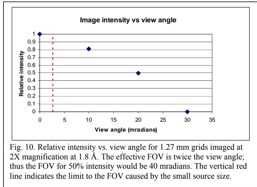
Fig. 10. Relative intensity vs. view angle for 1.27 mm grids imaged at 2X magnification at 1.8 Å. The effective FOV is twice the view angle; thus the FOV for 50% intensity would be 40 mradians. The vertical red line indicates the limit to the FOV caused by the small source size.
