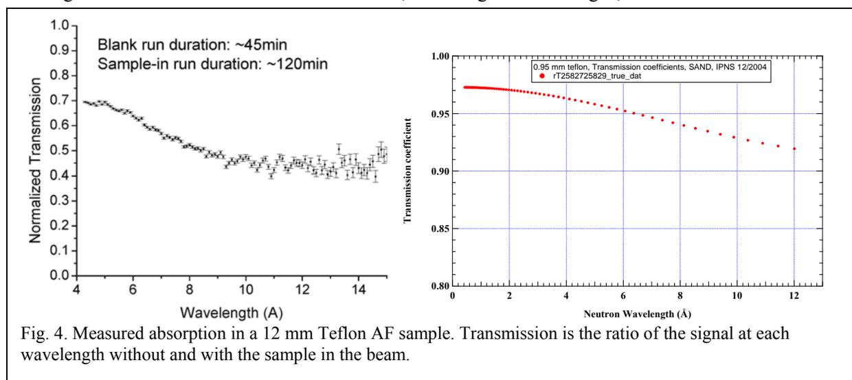
Fig. 4. Measured absorption in a 12 mm Teflon AF sample. Transmission is the ratio of the signal at each wavelength without and with the sample in the beam.
