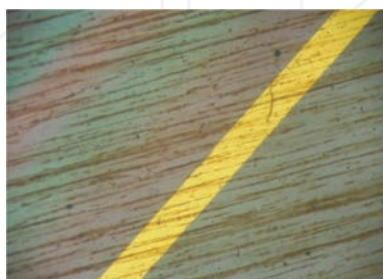
Figure 12. Microscopy image of 0.016 wt.% SWNT- \text{COOH} , 0.016 wt.% \text{Fe}_2\text{O}_3 in DI water. At 8 min, the internal reference is 30 \mu\text{m} . From Ref. [70].
