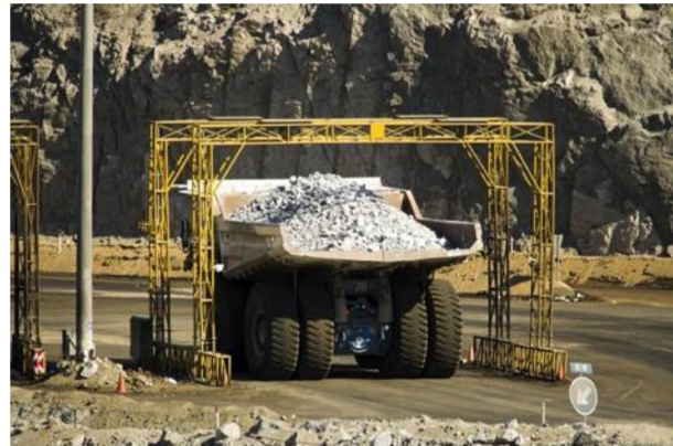
Figure 6: Gamma-ray detectors for sorting ore
