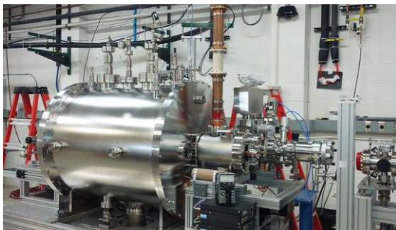
Figure 1: Electron gun installed in vault.
