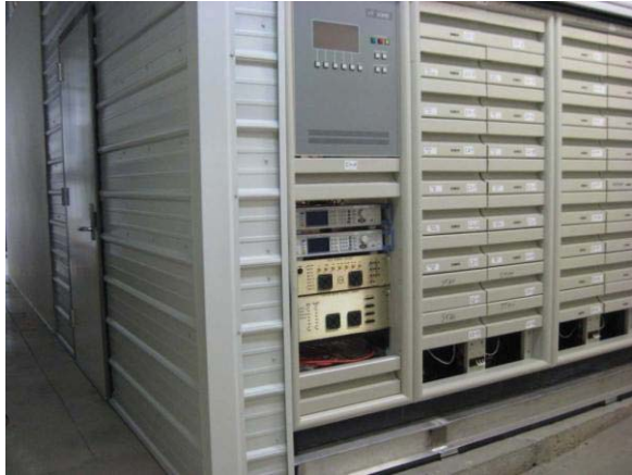
Figure A4. RF Power amplifier and low level control modules.
