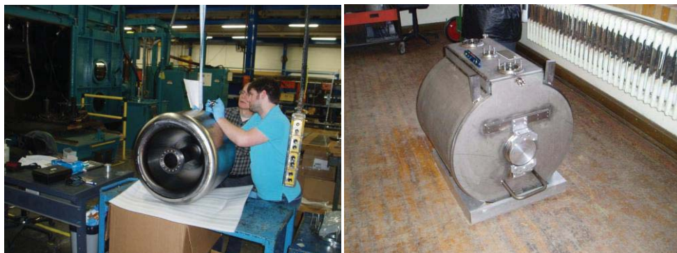
Figure A2. Niobium SRF gun cavity in preparation for last e-beam welds (left) and helium vessel after integration with cavity (right).
