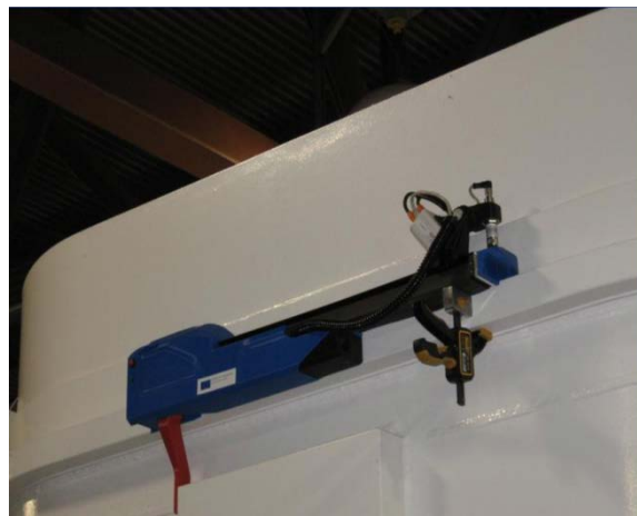
Figure 2.13. LMCV scanner attached to cask
