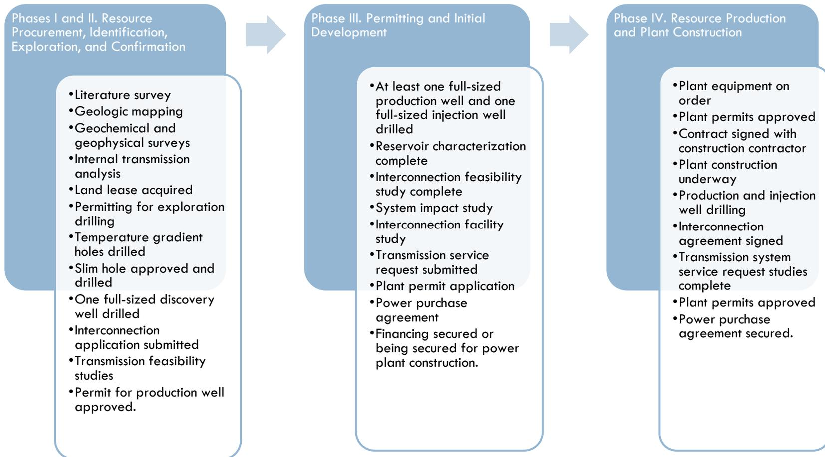
**Figure 1. U.S. Geothermal Energy Association’s terms and definitions for geothermal resource development (2010a)**
