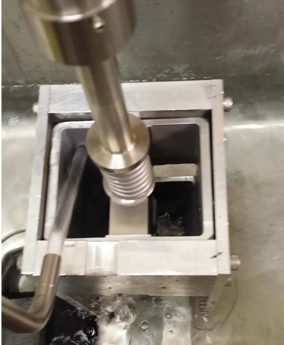
Figure 3.24 Water Impingement in Mockup Test with Upper Part of Fuel Element
