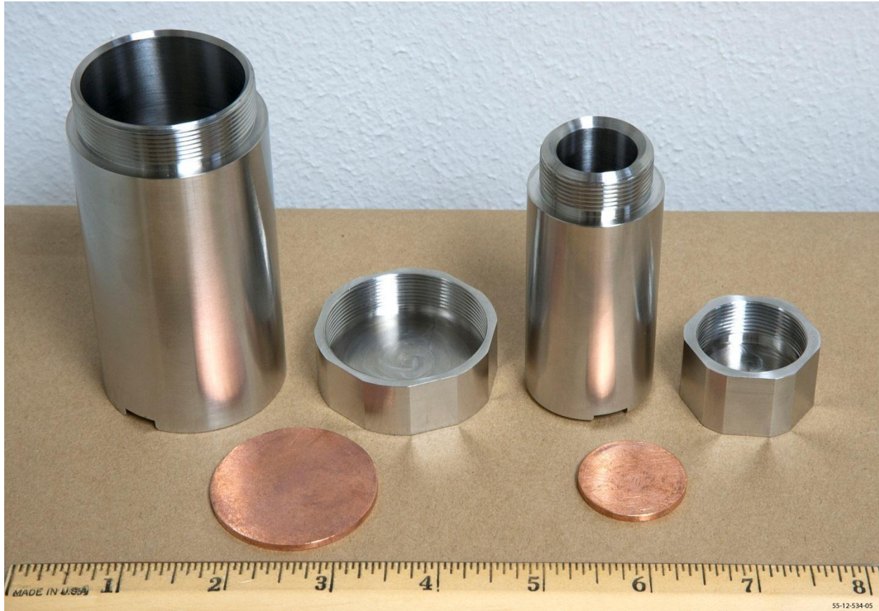
Figure 1. Photos of LANL prototype “middle” and “inner” containers with lids removed.
