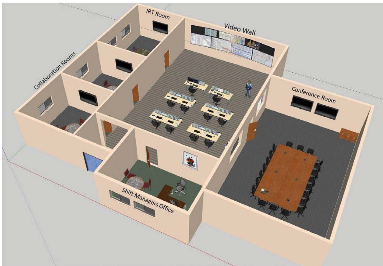
Figure 17. A recommended AOCC layout.
