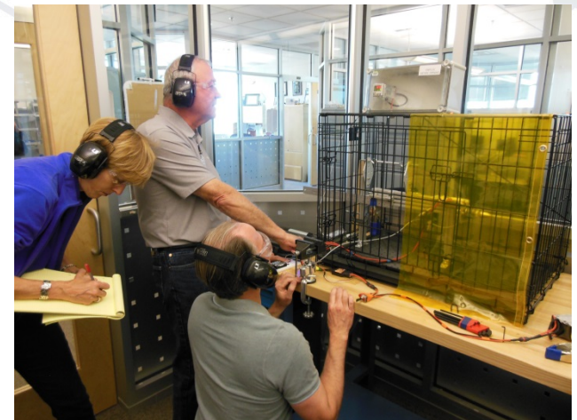
Judges do experiments to estimate lift vs RPM of quadrotor motor and propeller
