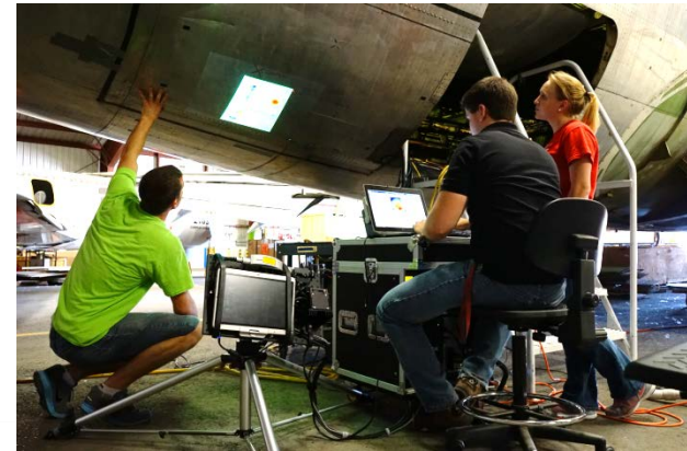
Acoustic Wavenumber Spectroscopy identifying damage in 737 fuselage
