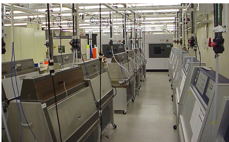
Figure 8.) 3M's Accelerated Weathering Chambers (Light, Heat, Water Spray)
