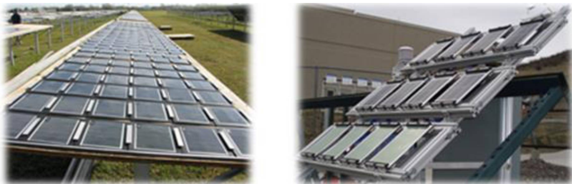
Figure 9.) Outdoor Testing of Ultra Barrier Top Sheets on Modules in Florida and Colorado
