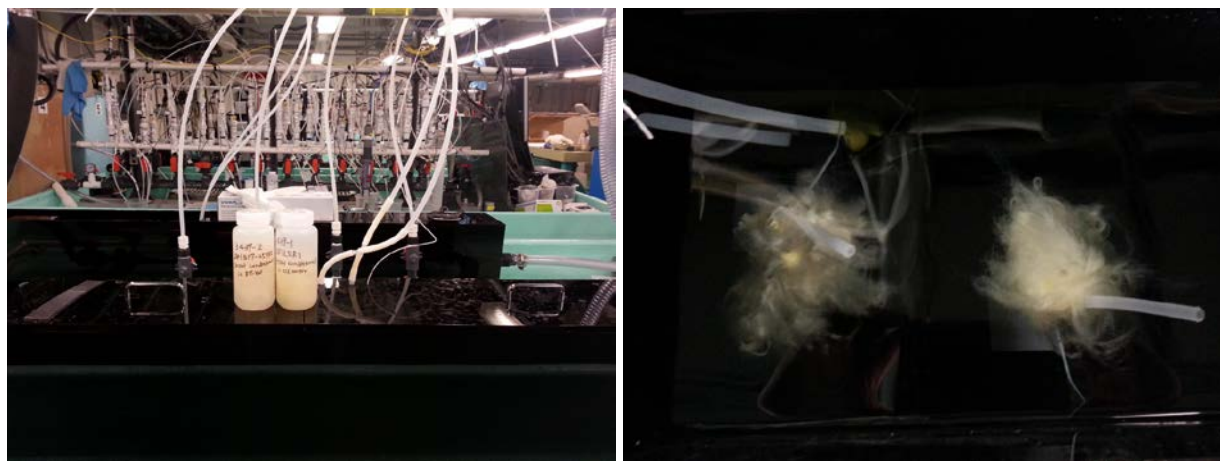
Figure 14. ORNL's braid and leno woven adsorbents after KOH conditioning (left) and after submersion in PNNL's flume on day one (right).
