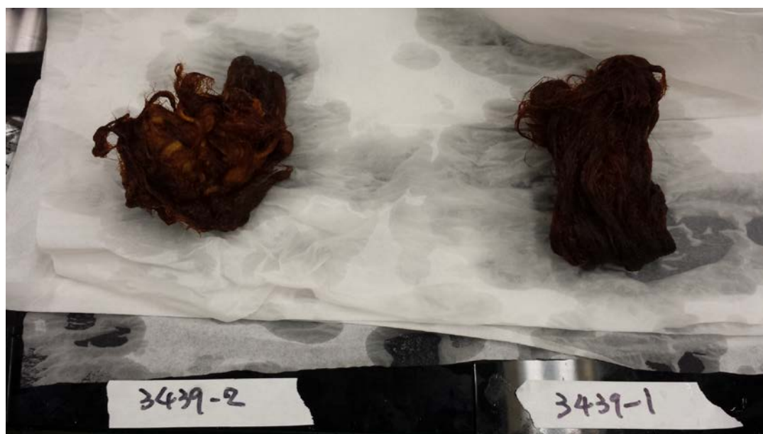
Figure 16. ORNL's AF1 braid and leno woven adsorbents after removal from flume.
