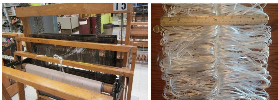
Figure 2. Leno weaving machine (left) and the L2 half leno single cloth made at Philadelphia University (right).
