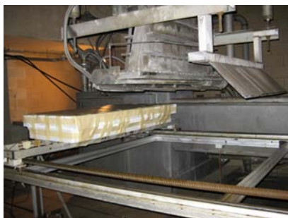
Figure 3. Electron beam set-up used for irradiating braids and leno woven fabrics.
