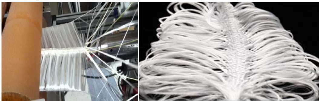
Figure 1. Braiding machine (left) and a representative braid made at Steeger USA (right).
