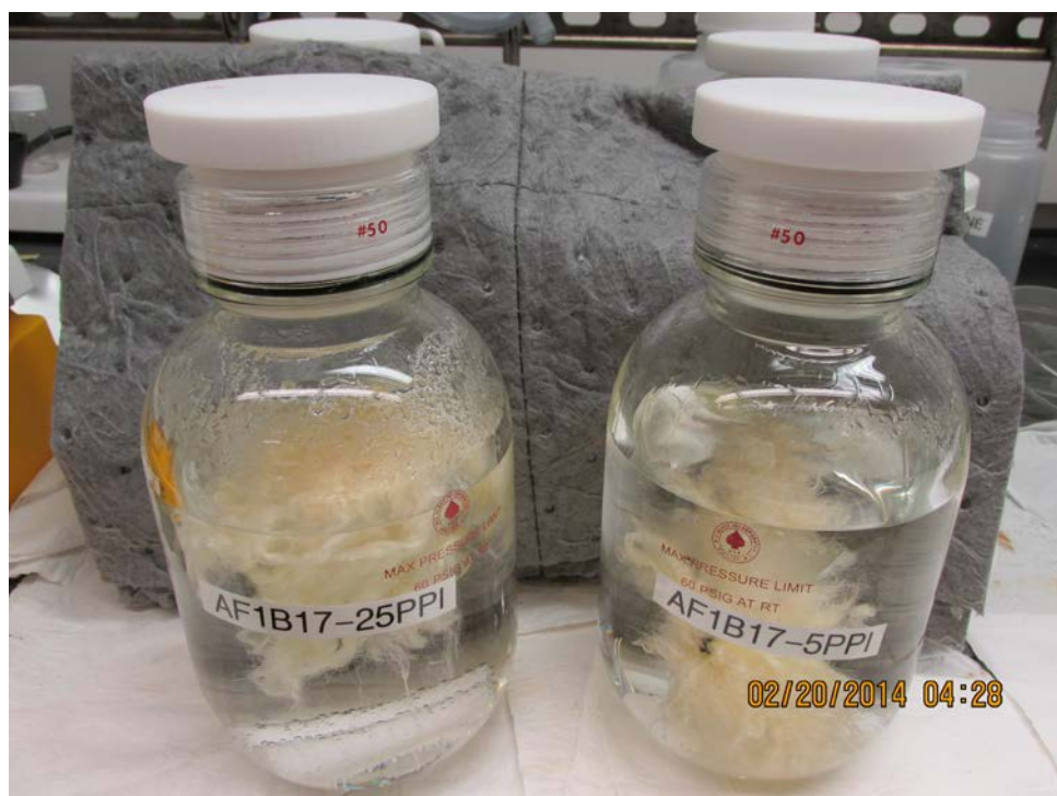
Figure 4. Braided adsorbents after amidoximation reaction.
