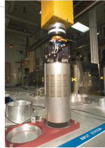
Long-Term Storage Container being measured on the Automated Non-Destructive Assay Instrument
