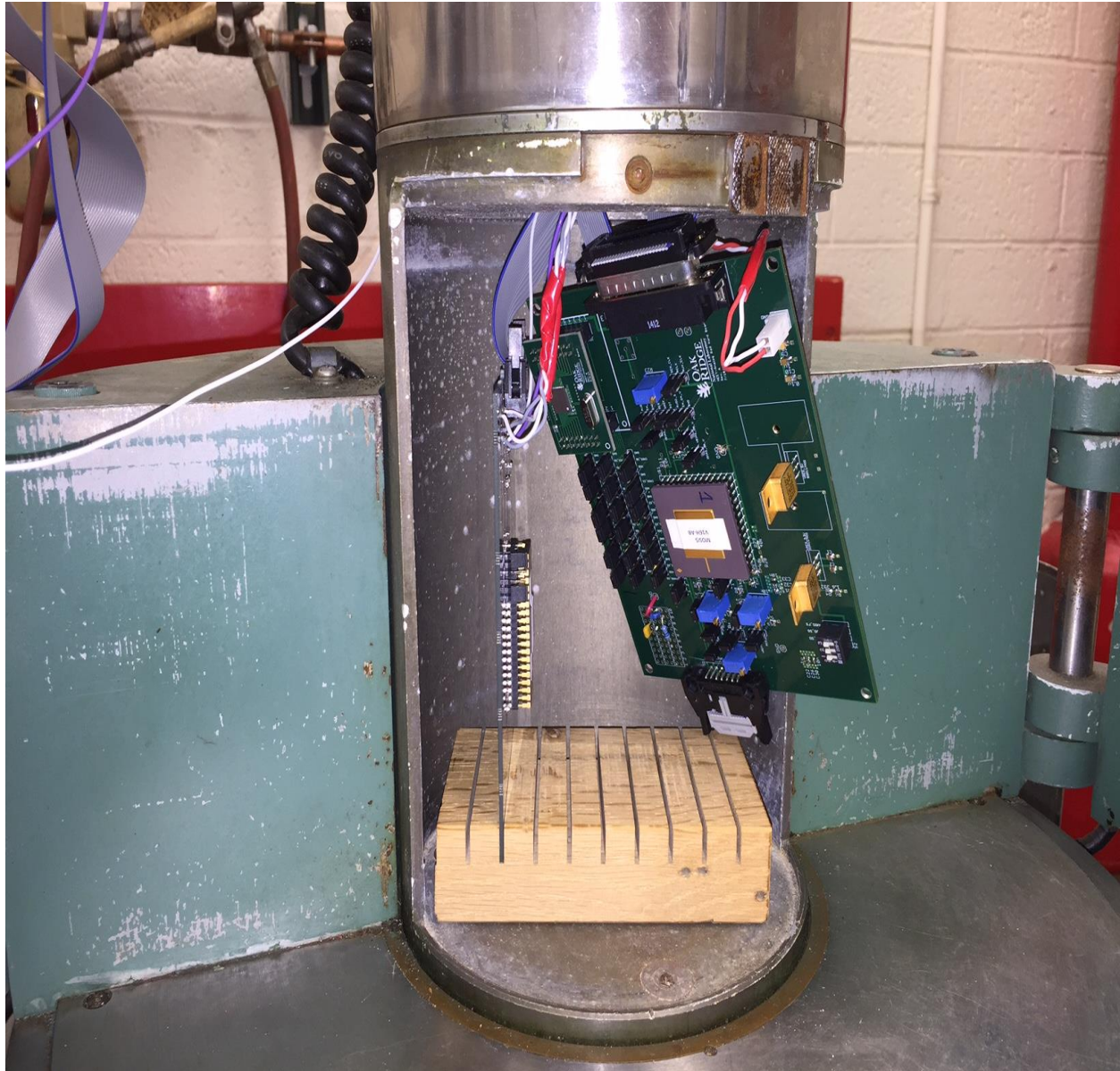
Fig. 21. Rad-hard board setup before test commencement.
