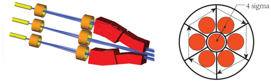
Figure 12: Schematic of the funnel with three channels shown (left); cross section of the funnel magnet – red circles represent the bunches (right).
