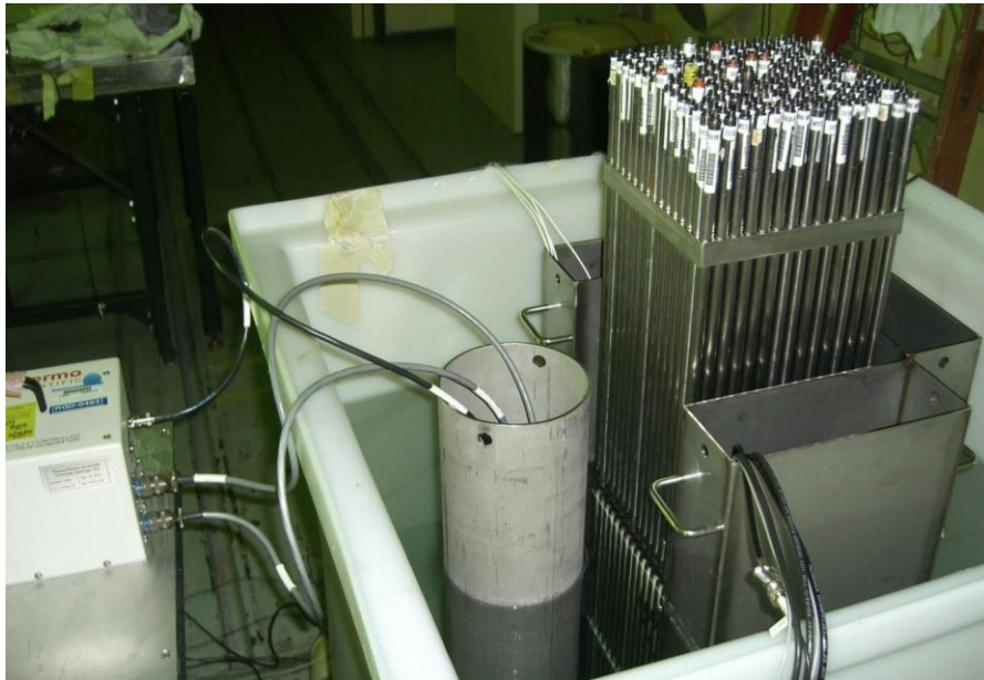
Figure 1. The DDA experimental setup includes a DT neutron generator inside a stainless steel pipe, a 15x15 fresh fuel assembly, and three stainless steel pods holding multiple ^3\text{He} detectors inserted into HDPE, Cd-wrapped sleeves.
