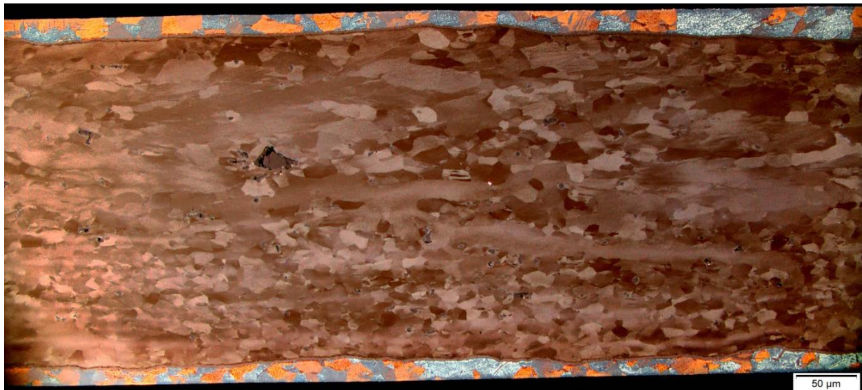
Figure 14. Example of Typical Surface Roughness at the Interface between Zr and U-10Mo (Edwards et al. 2012)
