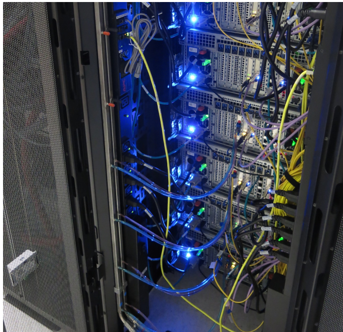
Figure 4: Image of the manifolds mounted in rack. Orange and black rubber caps block off the stub outs not in use.
