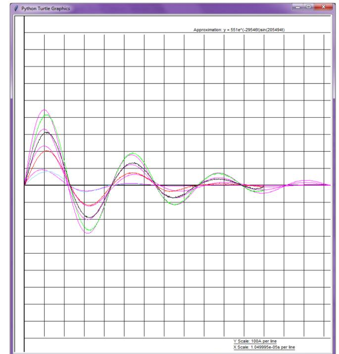
In addition to the previous plot, I also developed an algorithm to create an equation to approximate the current data (current versus time). These ringdowns do not have a burst, they just oscillate, and their peaks decay exponentially. From the derived equation, the RLC values of the fireset can be calculated. The above graph shows four different ringdowns of four different capacitor voltages for one detonator.
