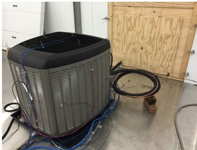
Fig. 16. Variable-speed unit B outdoor unit installed in environmental chamber.
