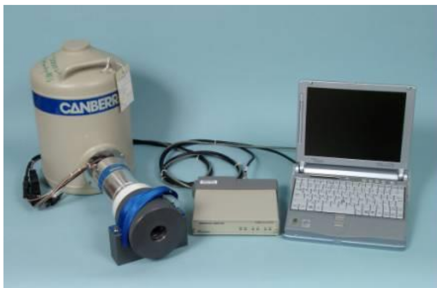
Fig. 1. Detector system setup for plutonium isotopic measurements.
