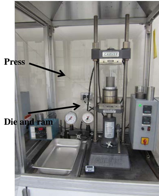
Figure 1: Carver press utilized for natural \text{UO}_2 pellet fabrication.
