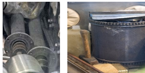
Figure 5. DMO furnace tubes, augers, and basket
