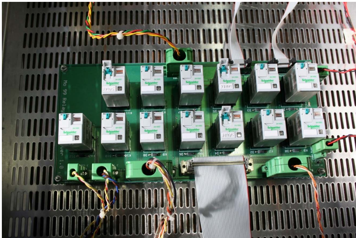
Figure 15. Interlock chassis top view showing the PC board with relays.
