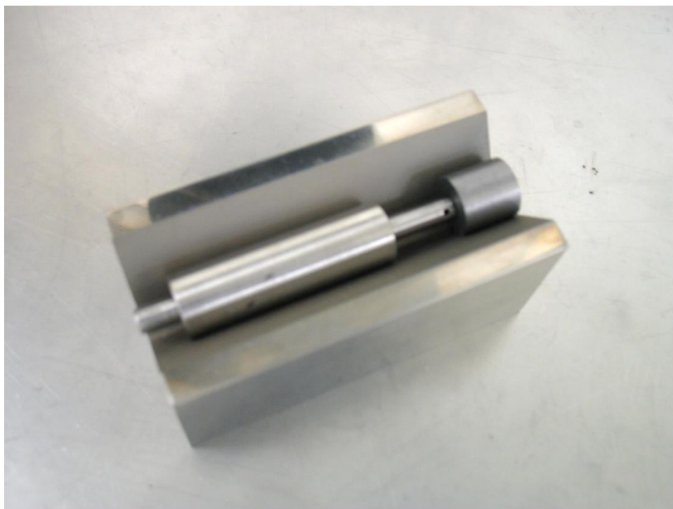
Figure 2. Compact epoxied to mounting rod in centering vee-block.
