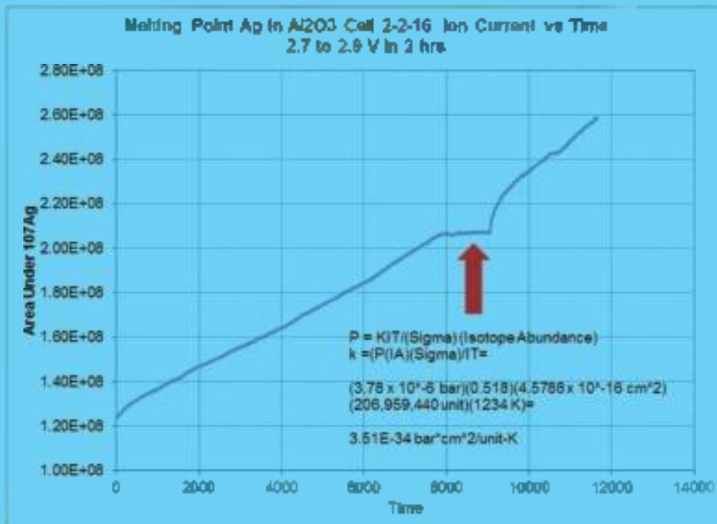
Figure 3: A sample calibration run resulting in the calibration curve and calibration constant  $k'$ . This experiment was Ag in Aluminum Oxide cell. The resulting factor is key to convert measured intensity to pressure.
