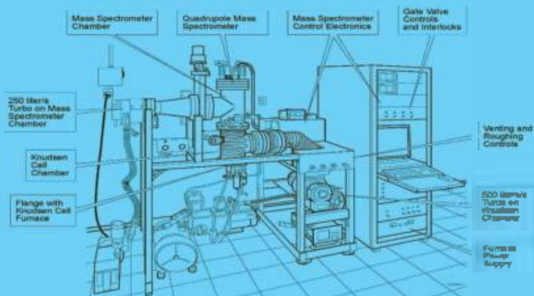
**Figure 2.** A detailed diagram of the KEMS system at NASA-Glenn (we are presently working in collaboration with Dr. Nathan Jacobson at NASA-Glenn).
