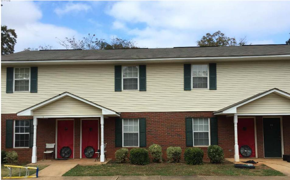
Figure 10. Configuration for guarded blower door test of center unit
