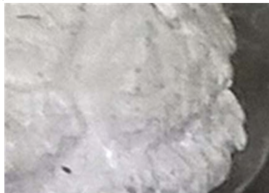
Figure 16. PS/POLYMER-BLEND-B/MMT-ABU foamed in pressure vessel. Foam density ~50kg/m 3 .
