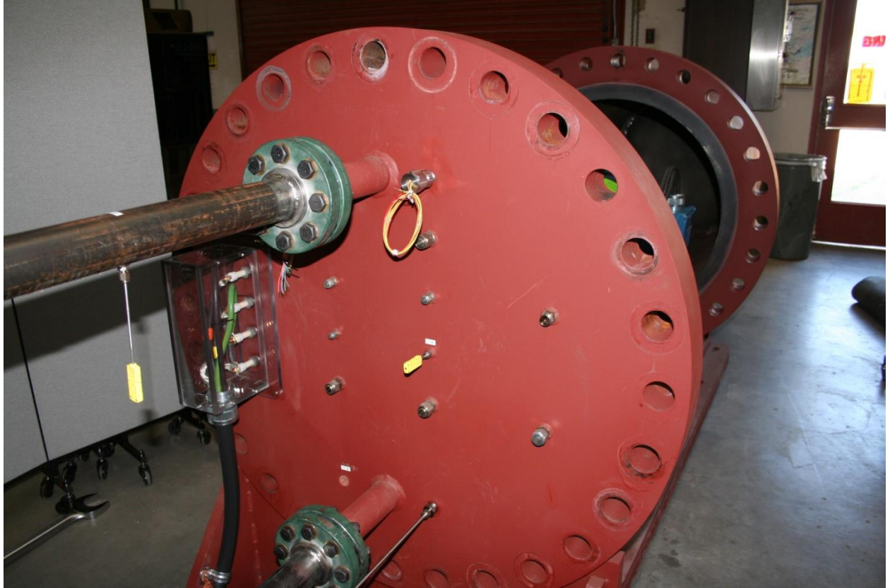
Figure 5. Fixed flange. Motor power inlet feed-throughs at center left. helium discharge pipe at the top, and return helium pipe at the bottom. Some instruments for temperature and accelerometers installed.
