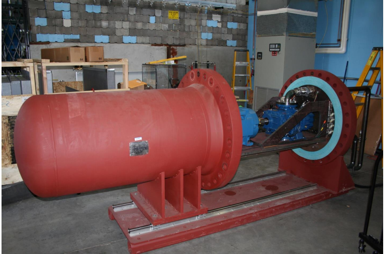
Figure 3. Vessel open, showing blower and motor.
