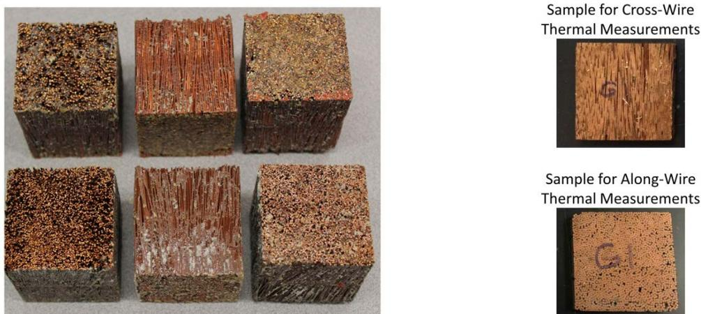
**Figure I-15: Winding sample blocks prepared by ORNL for thermal property measurements (left), cut samples prepared by ORNL and sent to NREL for directional thermal property measurements (right)**
