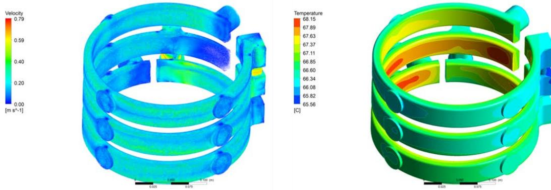
Figure I-4: CFD-generated plots showing the coolant velocities (left) and coolant channel temperatures (right).
