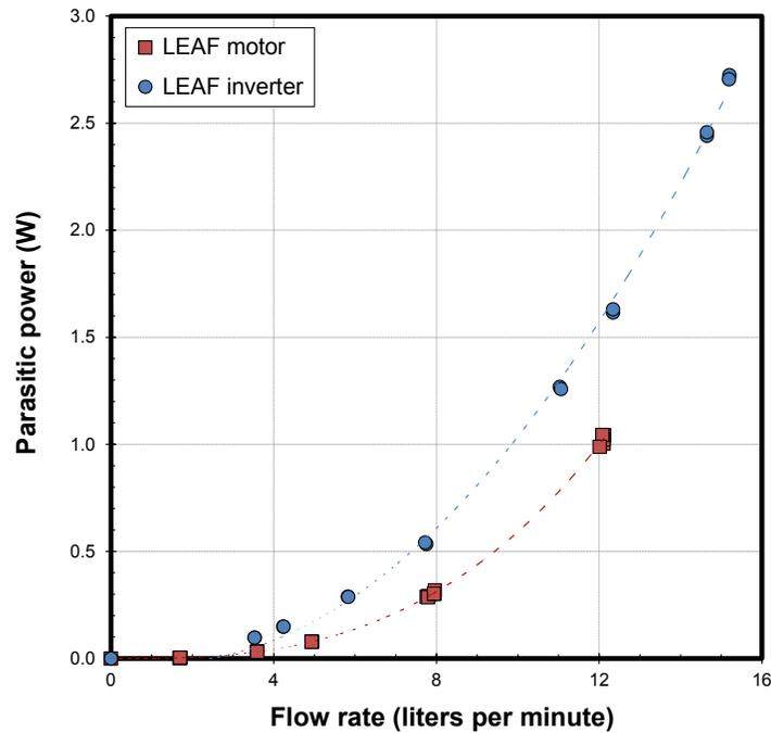
Figure I-12: Experimentally measured parasitic power losses for the Nissan LEAF motor and inverter heat exchangers
