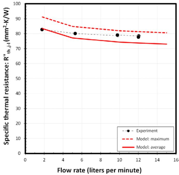
Figure I-9: Experimentally measured and model-predicted IGBT thermal resistance values for the 2012 Nissan LEAF inverter
