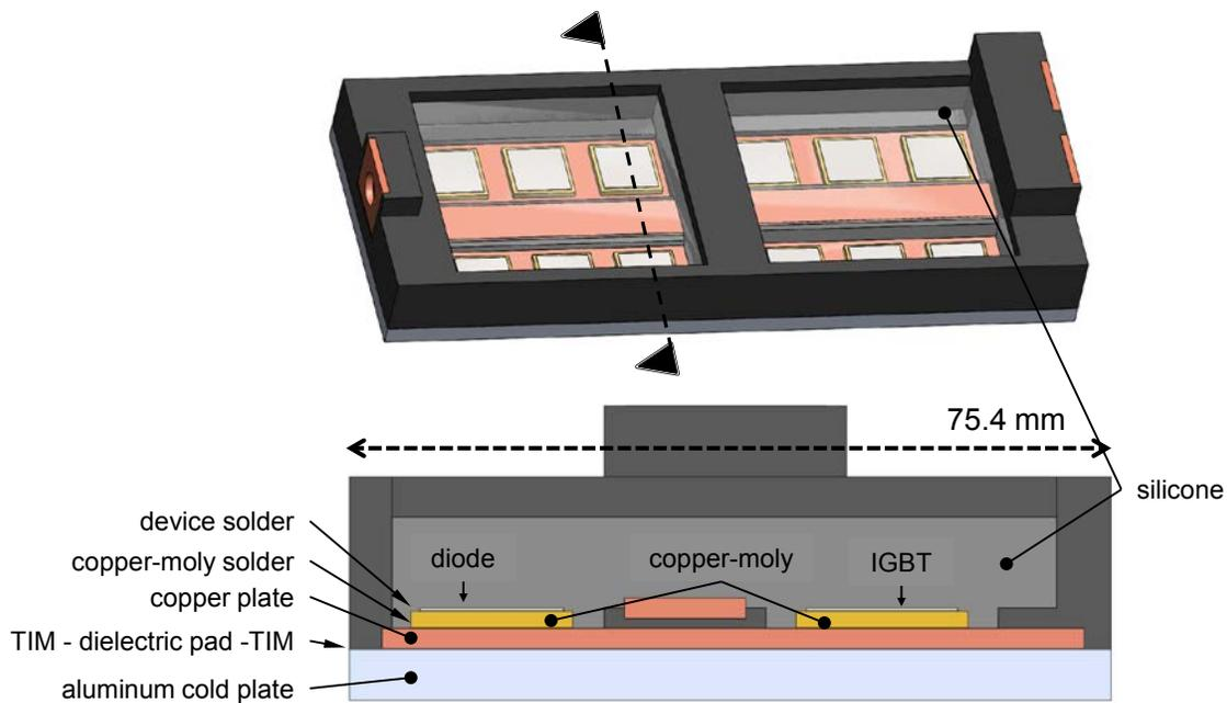
Figure I-8: CAD model of a Nissan LEAF power module. The various power module layers are shown in the lower, cross-sectional view.
