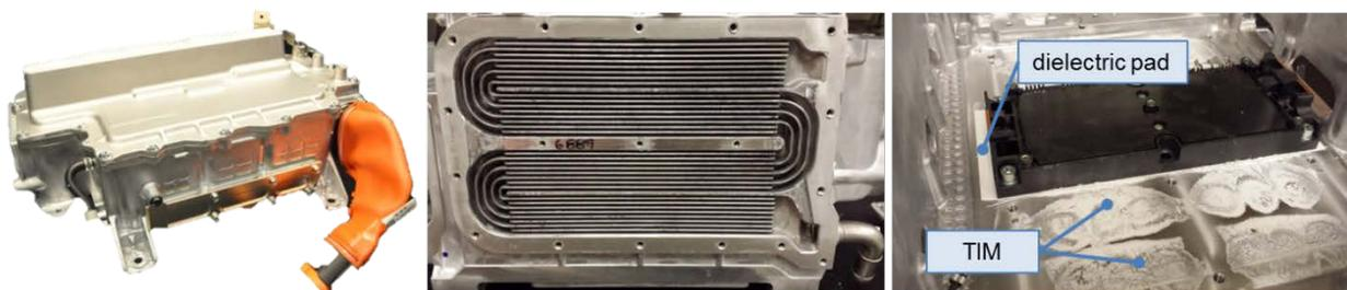
Figure I-7: Pictures of the 2012 Nissan LEAF inverter. The middle image shows the cold plate cooling channels. Image on the right shows one power module mounted on the cold plate. The dielectric pad and TIM layers are shown (right).
