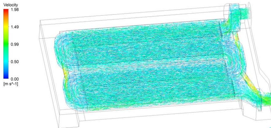
Figure I-10: CFD-generated plot showing the coolant velocity vectors at a flow rate of 10 Lpm
