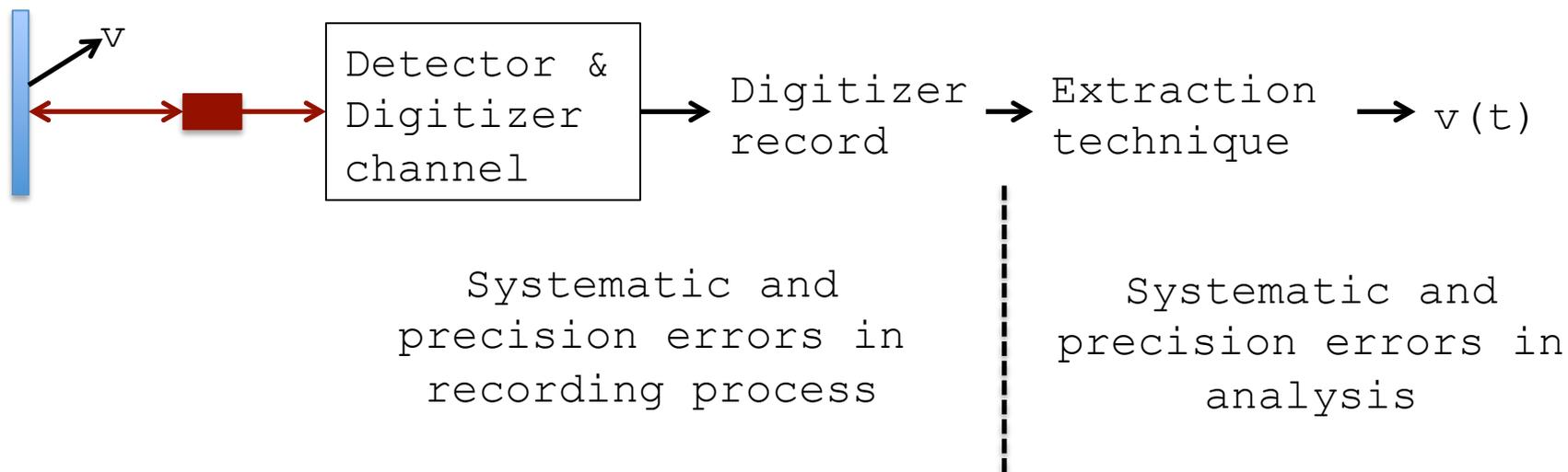
The error estimated from the analysis of the data can change with refinements in analysis technique. However, the accuracy and precision of the digitizer record are intrinsic to the measurement and will never change. The precision will reveal itself in split-signal experiments, but the systematic errors require a separate measurement of the detector response function.
