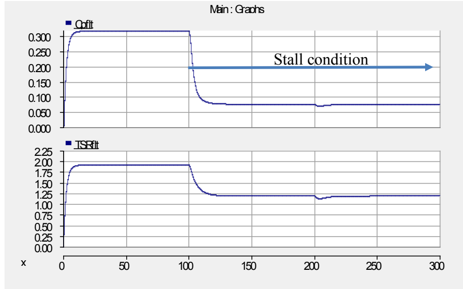
Figure 8. Operating C_p and TSR as the water flow changes in unstable operation
