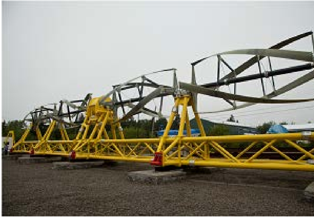
Figure 2. Example tidal generator consisting of series-connected Gorlov turbines
