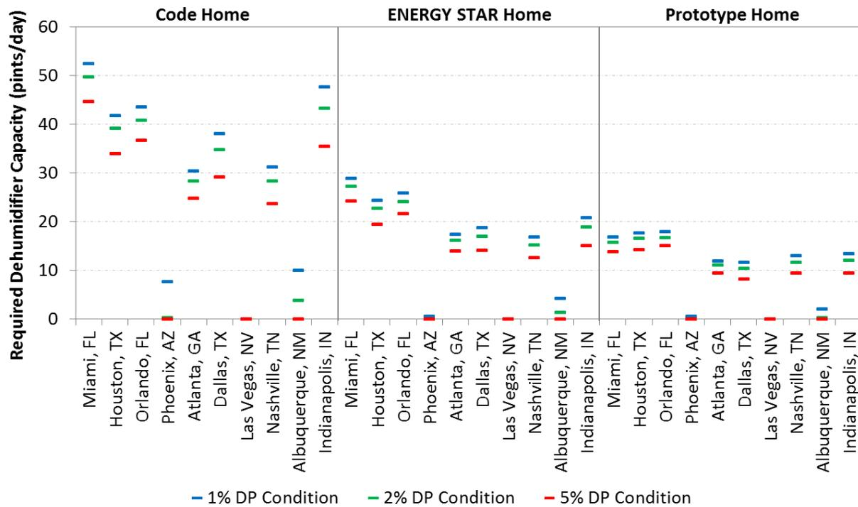
**Figure ES-1. Required whole-house supplemental dehumidification capacity based on different DP design conditions for three new construction house efficiency levels**
