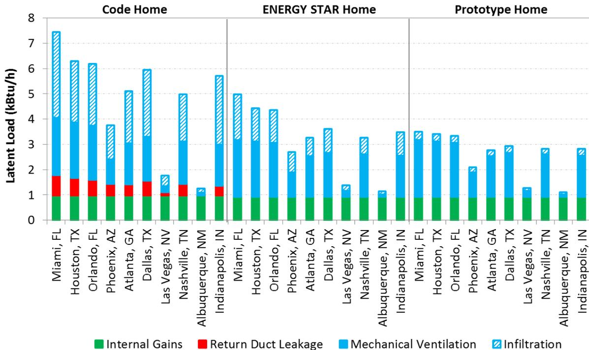
Figure 6. Total latent load breakdown at the 2% DP design condition
