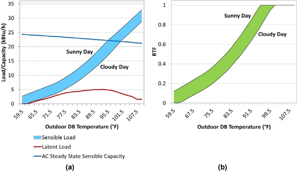
**Figure 2. (a) A typical building load profile based on outdoor DB temperature and (b) estimated air conditioner RTF for a typical new construction home in Houston, Texas**
