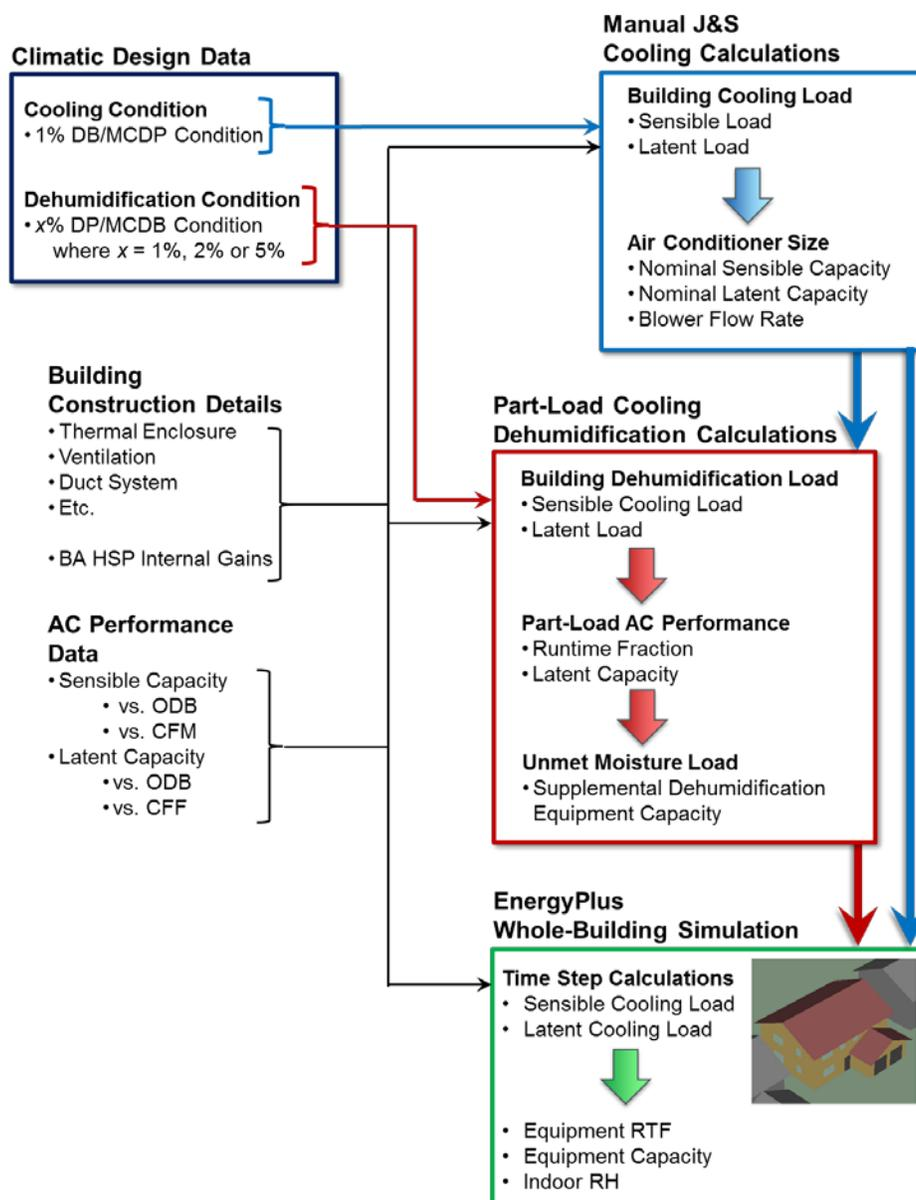
**Figure 5. Overview of the part-load cooling moisture load calculation and testing procedure**
