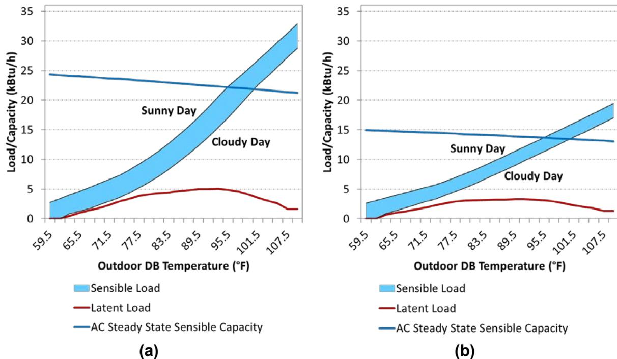
**Figure 8. Building load profile based on outdoor DB temperature for the (a) code home and (b) ENERGY STAR home in Houston, Texas**
