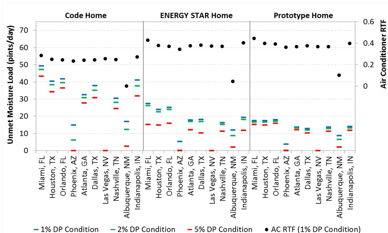
**Figure 10. Unmet moisture loads at 1%, 2%, and 5% DP conditions and air conditioner RTF (using Method 2); unmet moisture loads are higher than Method 1 (Figure 7)**
