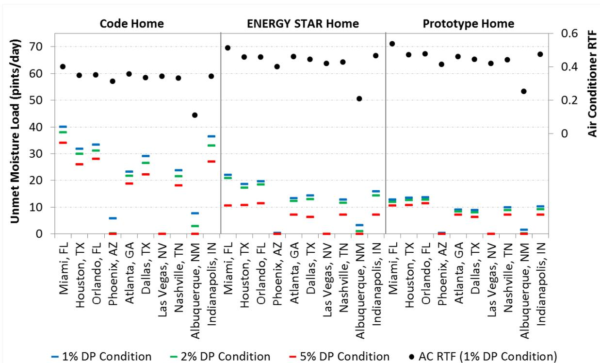
**Figure 7. Unmet moisture loads at 1%, 2%, and 5% DP conditions and air conditioner RTF (using Method 1)**
