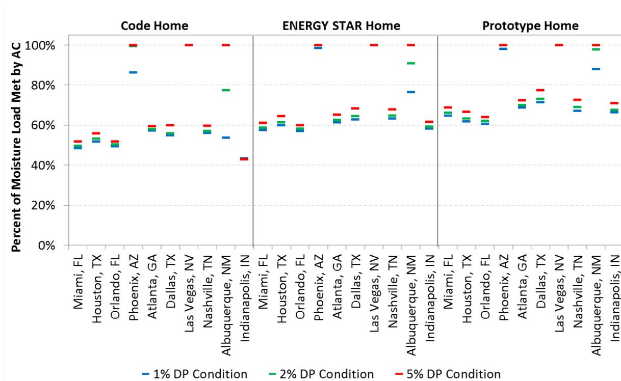
Figure 9. Percentage of the Method 1 moisture load removed by the air conditioner at 1%, 2%, and 5% DP conditions
