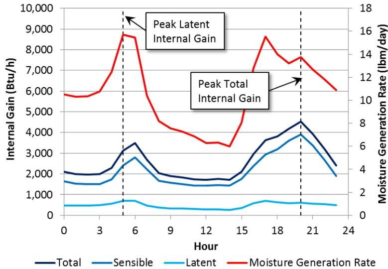
**Figure 4. Hourly internal gain profiles for the code home**
