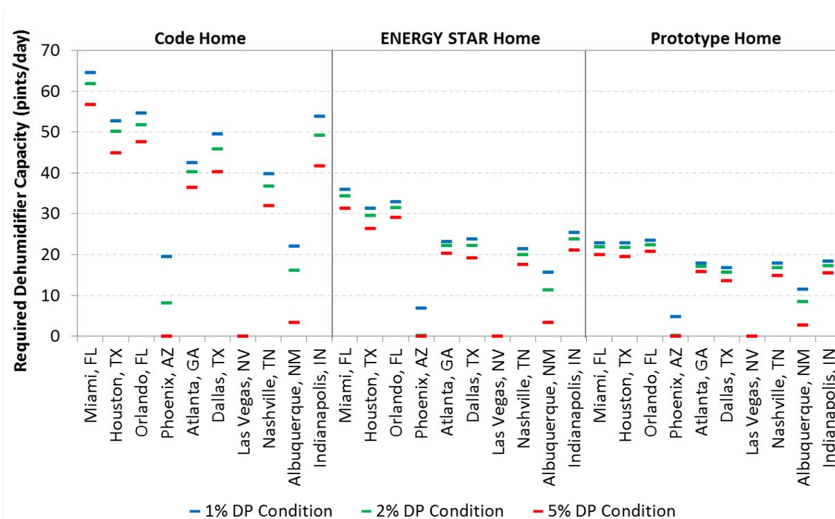
Figure 12. Estimated rated dehumidifier capacity required to meet the unmet moisture load from Figure 10 (Method 2) using 1%, 2%, and 5% DP conditions
