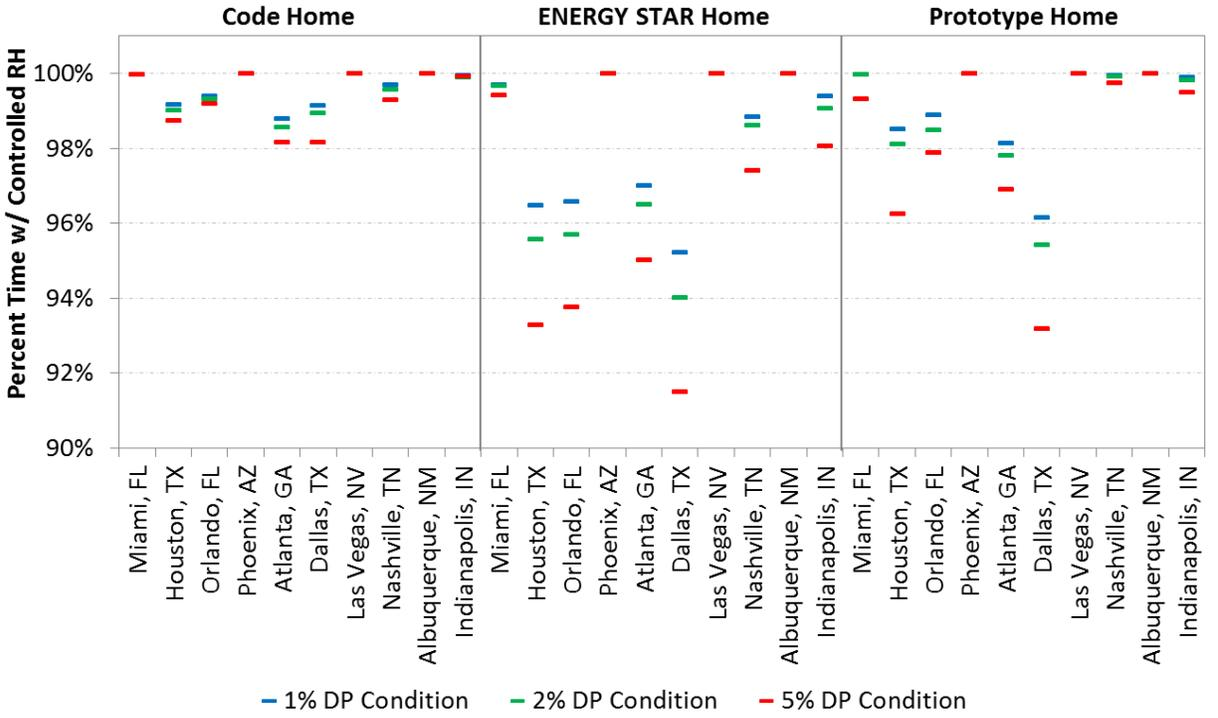
**Figure 13. Dehumidifier simulation results when sized based on 1%, 2%, and 5% DP conditions using the Method 1 sizing procedure (Note y-axis minimum value of 90%)**
