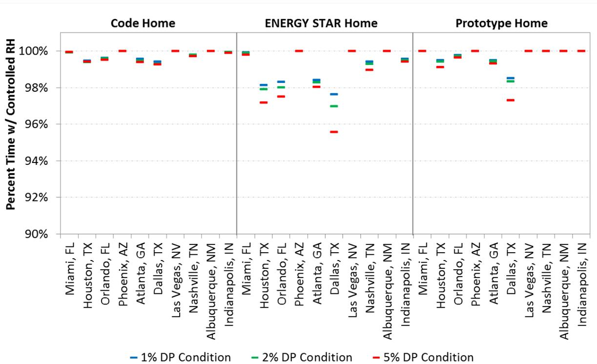
**Figure 14. Dehumidifier simulation results when sized based on 1%, 2%, and 5% DP conditions using the Method 2 sizing procedure (Note y-axis minimum value of 90%)**
