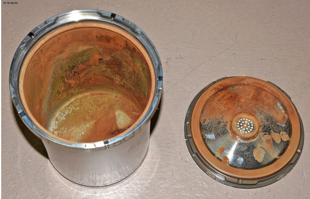
Fig. 2: SAVY container with interior corrosion.
