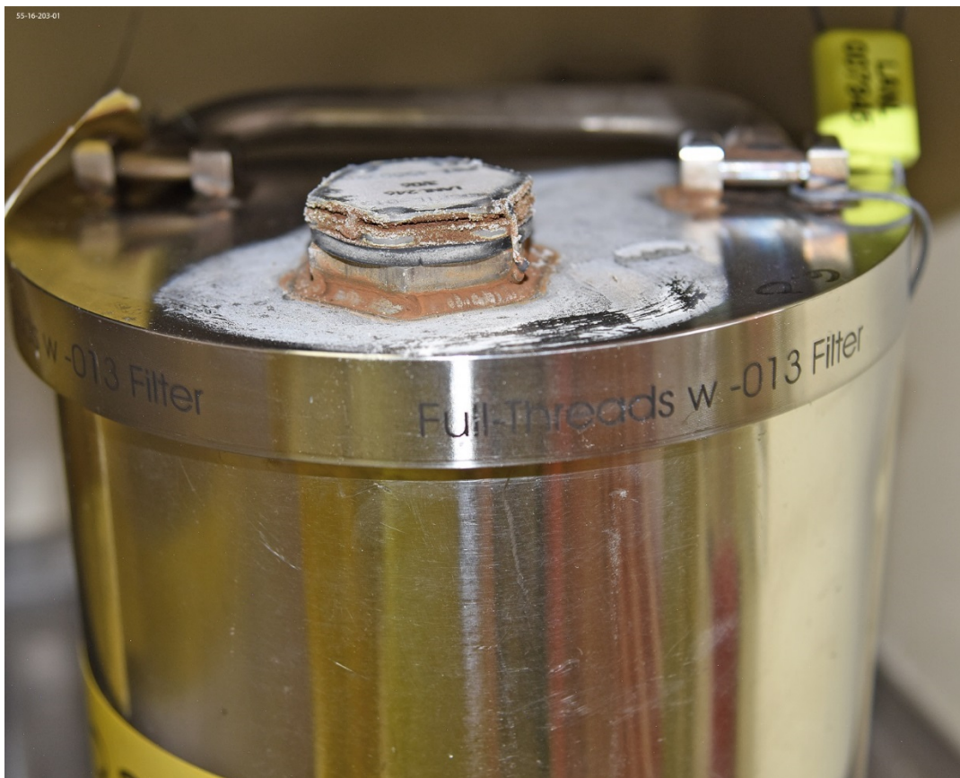
Fig. 1: Hagan canister with unacceptable corrosion levels.
