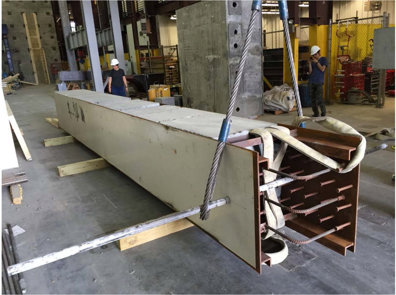
Figure 6-6. CA-20 module rotated into the horizontal position.
