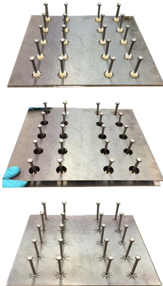
Figure 4-4. Steel plate and stud matrix.
