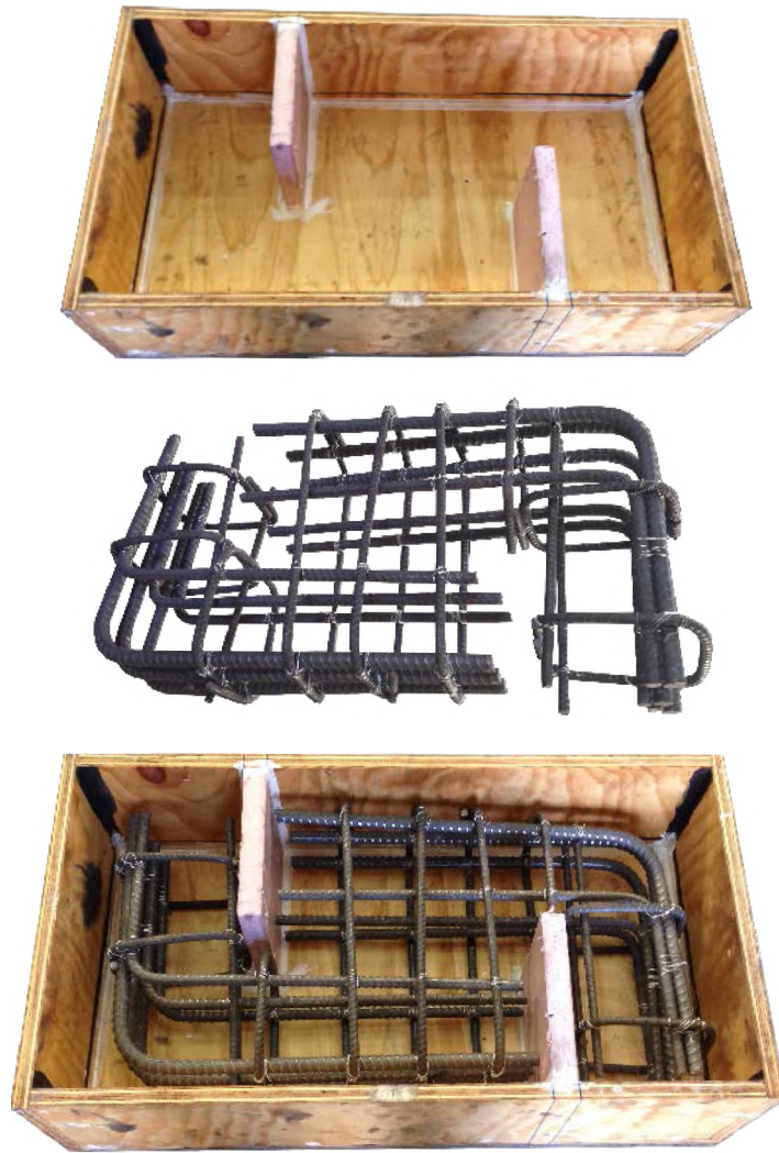
Figure 4-7: Monolithic Specimen Prior to Casting
