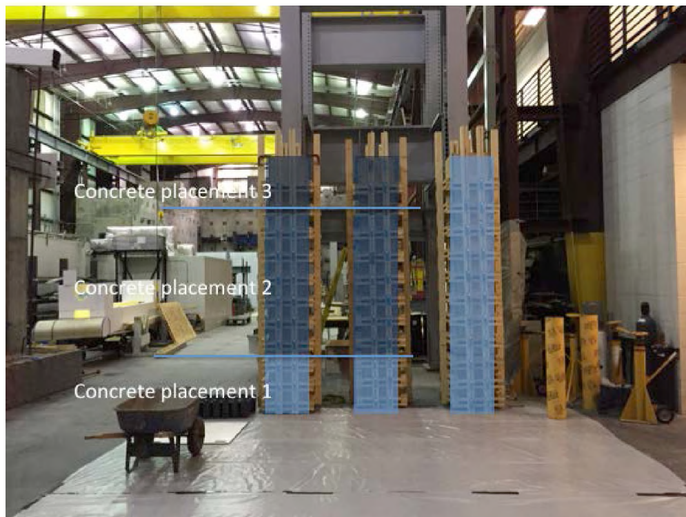
Figure 5-6. Concrete placement for Task 3 specimens.
