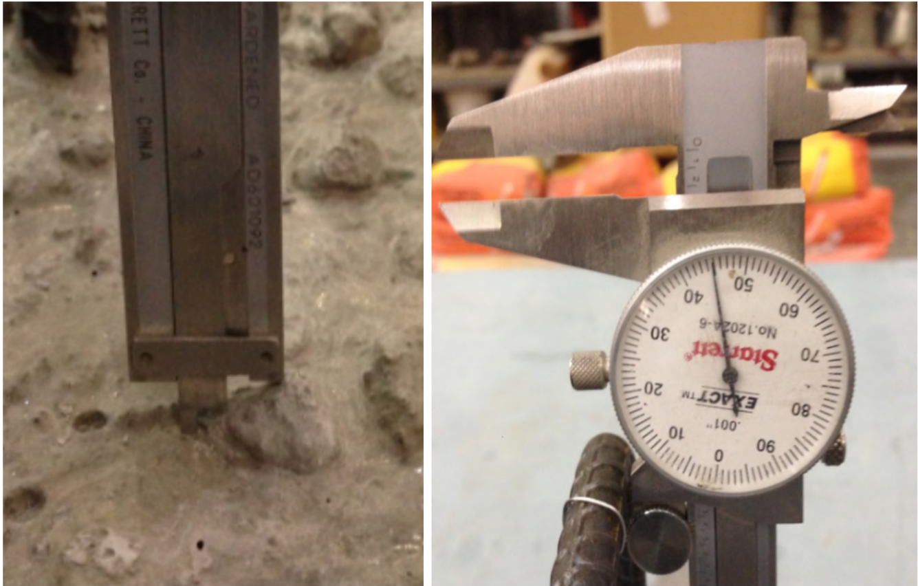
Figure 5. Roughness quantitative measurements
