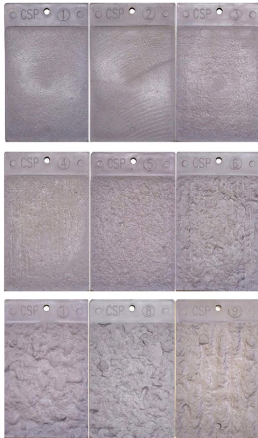
Figure 3-16: ICRI's standard CSPs
