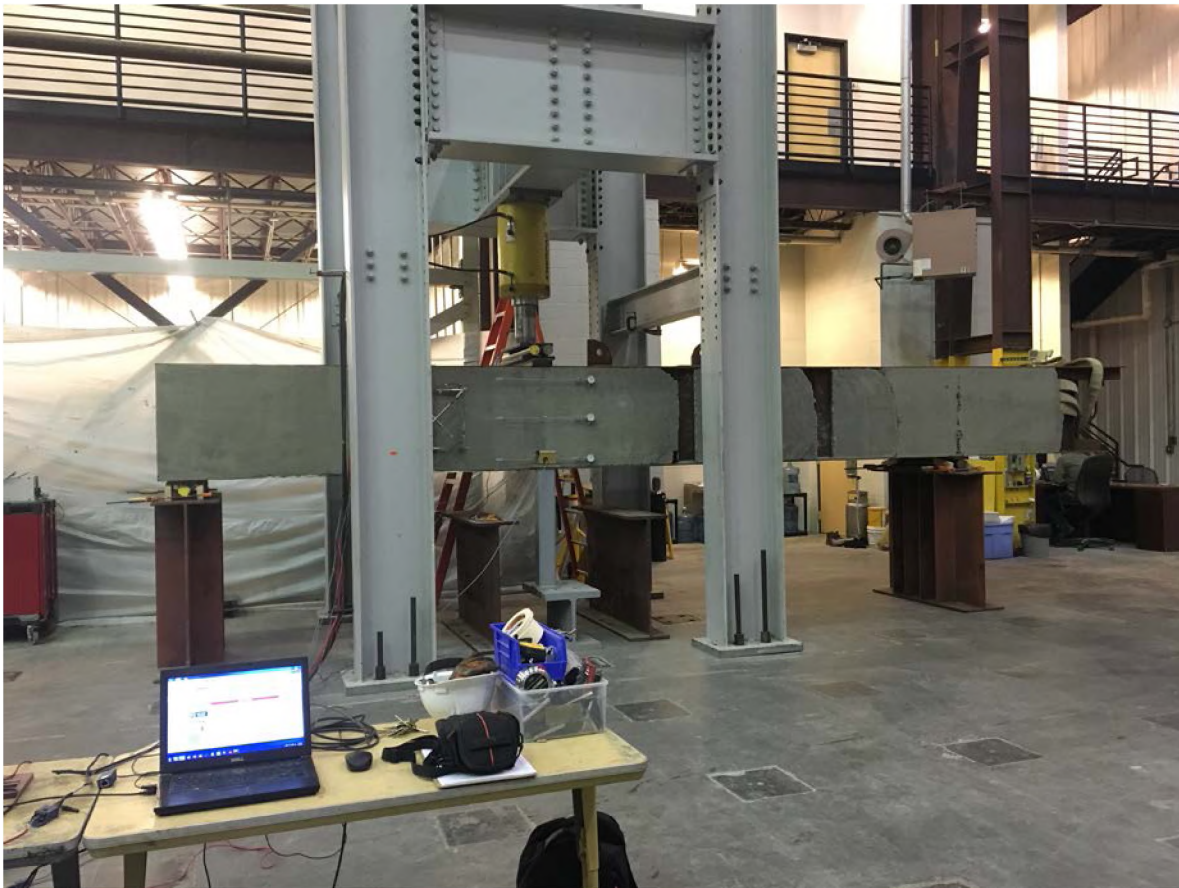
Figure 6-9. Task 4 specimen in test frame.
