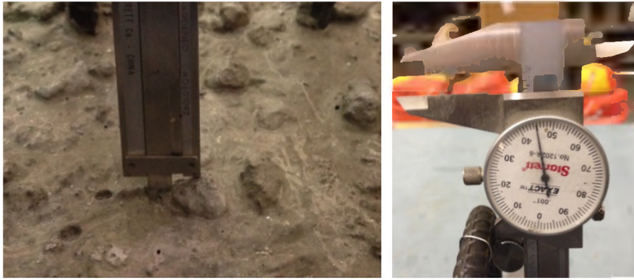
Figure 3: Roughness quantitative measurements.
