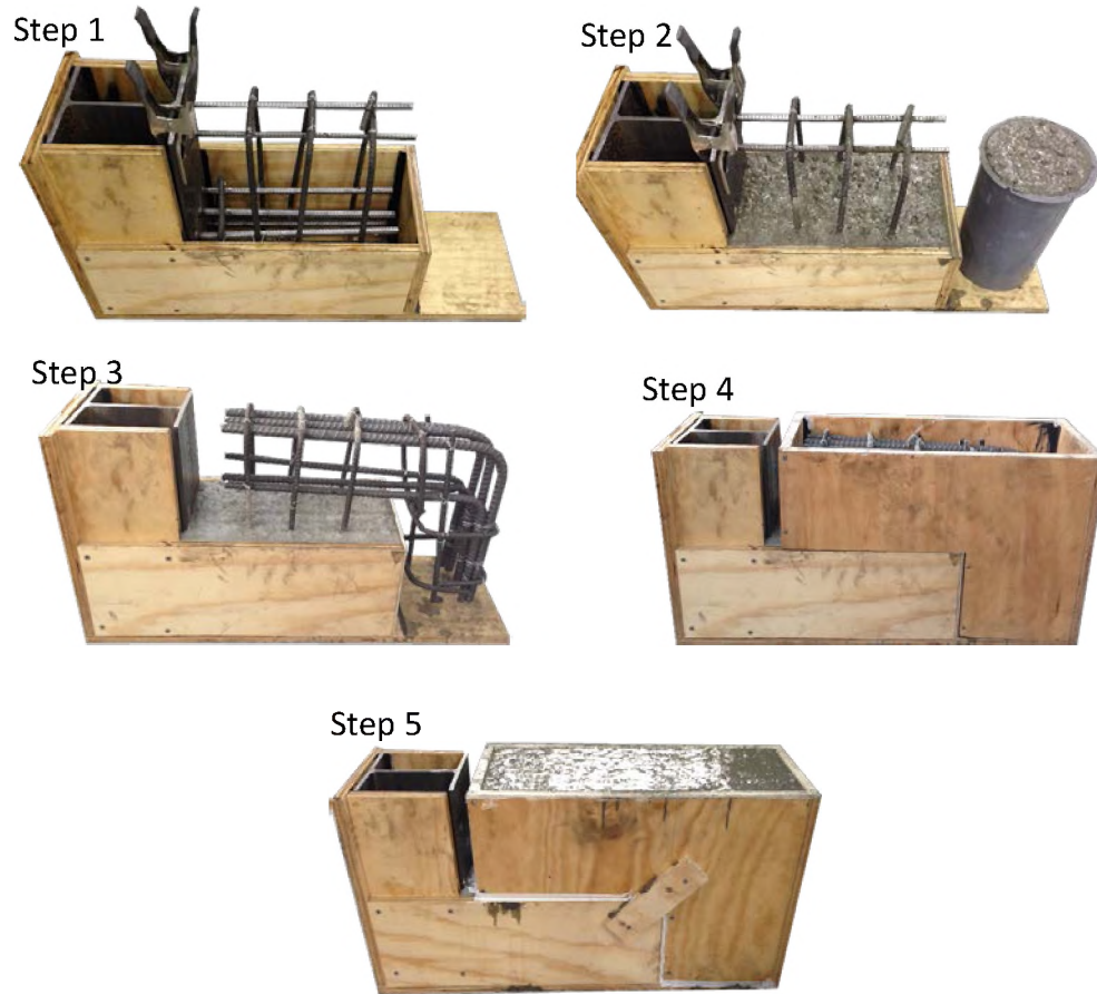
Figure 4-9: Cold-joint Specimen preparation
