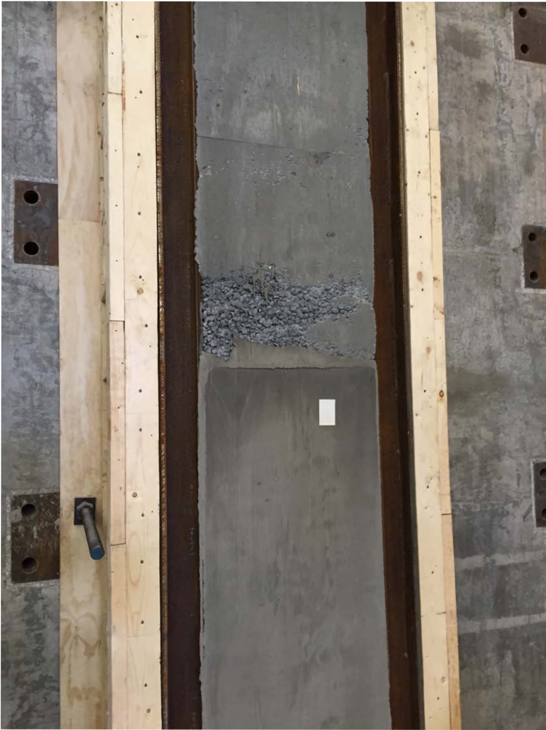
Figure 6-7. Segregation in SCC due to excessive slump.
