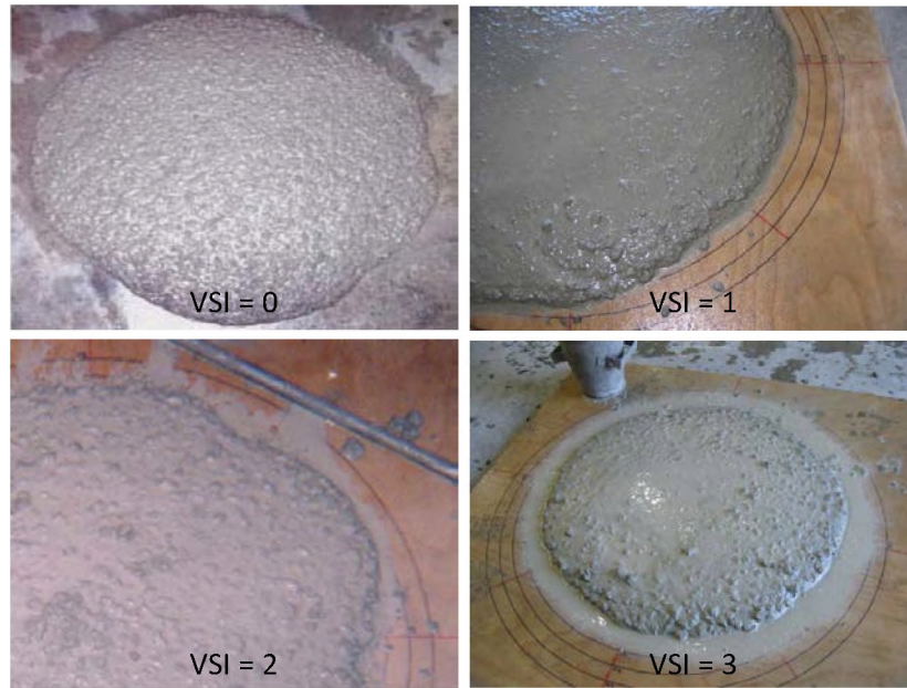
Figure 3-10: Visual stability index examples for various slump flow test
