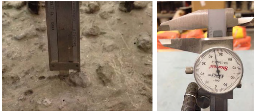
Figure 3-17: Roughness quantitative measurements
