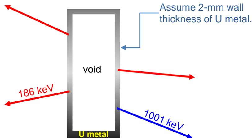
At our detector we see the *same amount of 186-keV* gammas for both cases above. But we see less of the 1001-keV gammas in a relative sense from the thin-walled box than the solid block.
