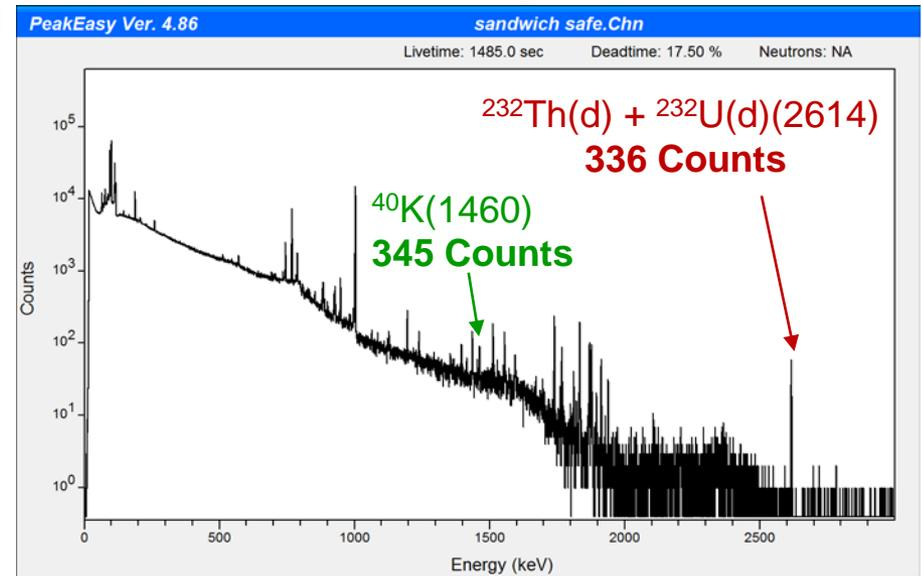
In the shielded (recycled) HEU case, the ratio of 2614:1460 counts is  $\sim 1:1$
