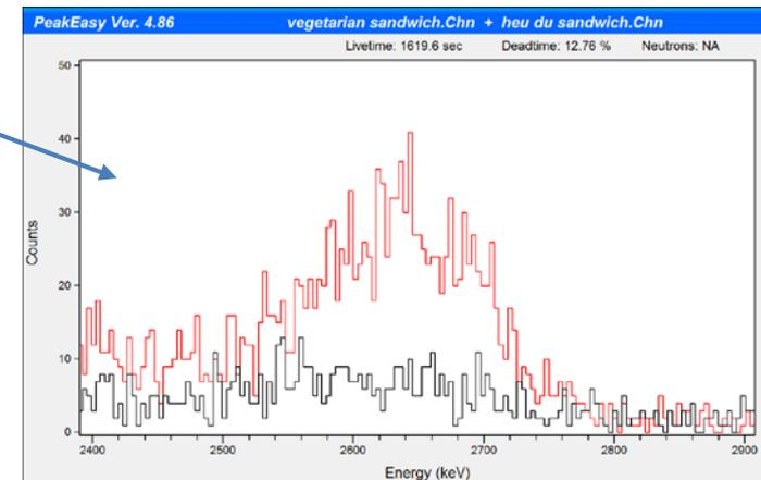
Without intrinsic radiation such as with the LaBr3 detector, the NaI spectra, clearly show the enhanced 2614-keV peak.
