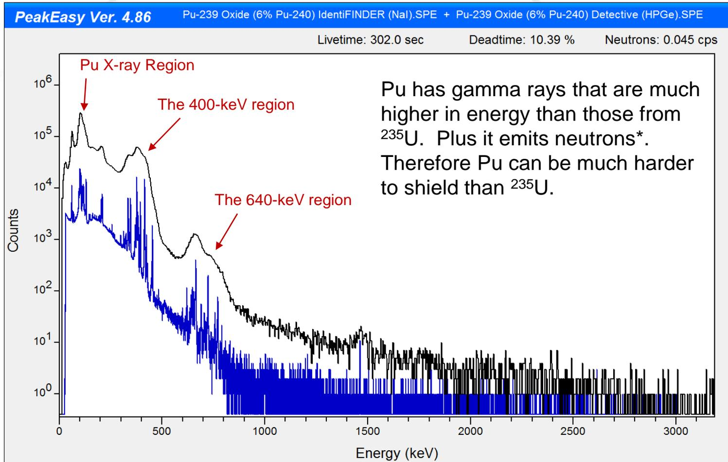
\* The mass for this Pu item is only 10g so the neutron signal is weak.
