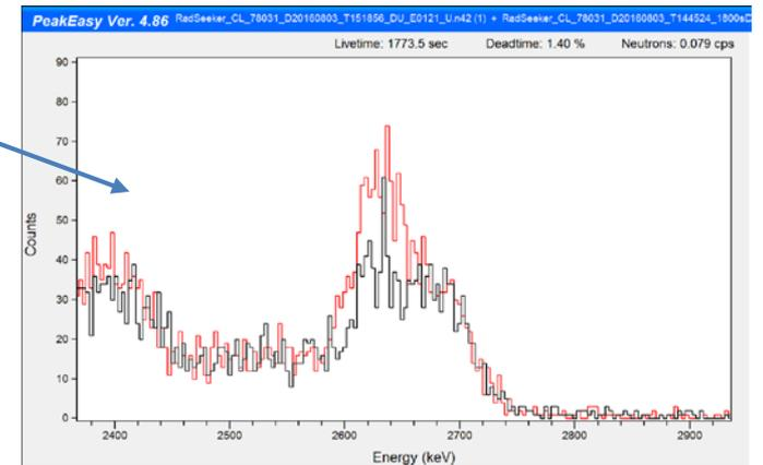
The intrinsic radiation from the LaBr3 detector crystal makes the presence of an enhanced 2614-keV peak more subtle than for other detector types.
