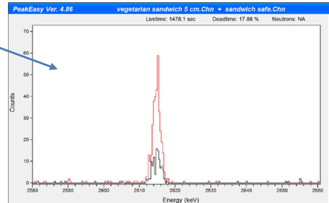
The superior peak-to-Compton ratio of the HPGe detector used to take these spectra further emphasizes the enhanced 2614-keV peak.
