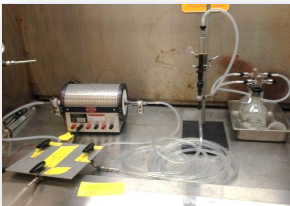
Fig. 3 System set-up for AlN pellet
