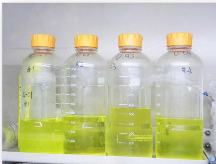
Fig. 11. Batches of U-234 solution following additional separation of Pu.
