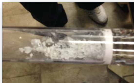
Fig. 4 Crushed AlN in quartz tube after heating.
