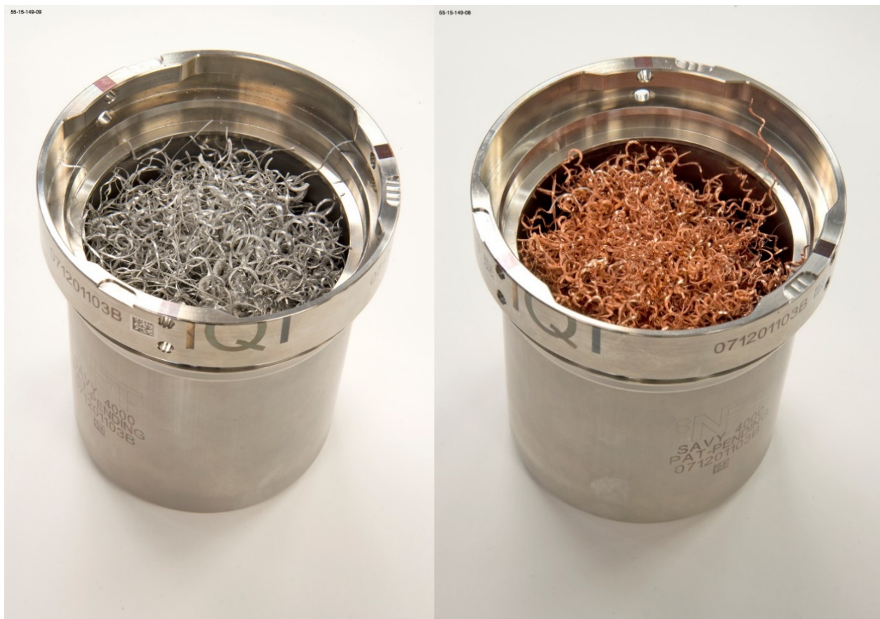
Figure 7: 500 grams of Pu equivalent volume compacted into one quart Savy containers.
