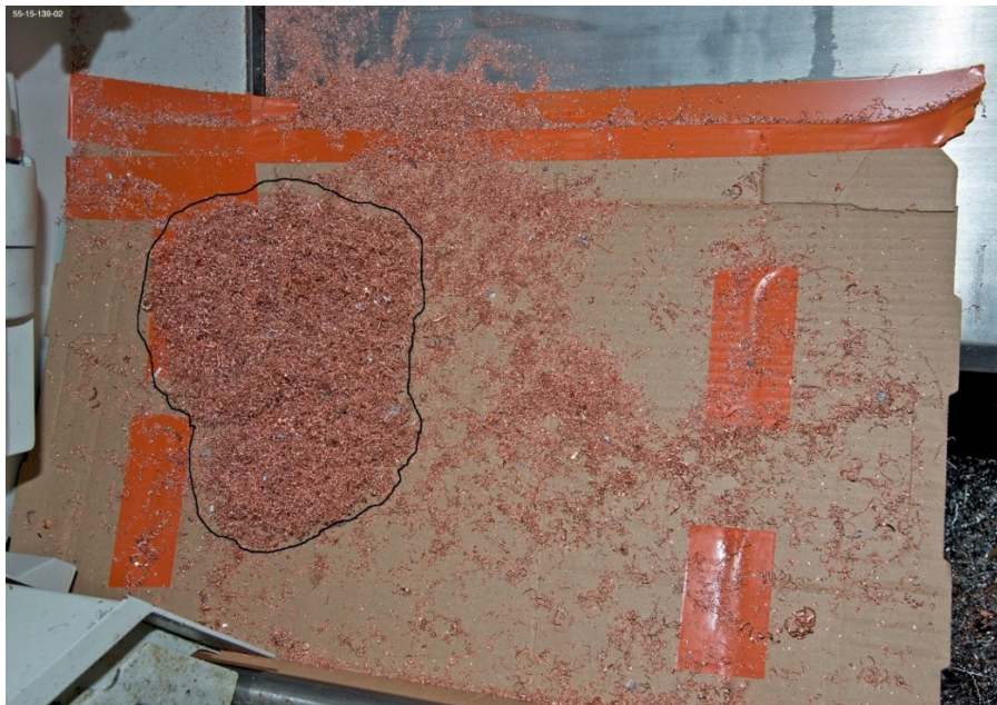
Figure 1: T-base 2 machined turnings (bird nest turnings pile)
