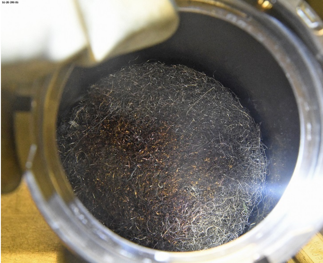
Figure 8: 100 grams of Pu turnings produced on the Precitech in a one quart Savy container
