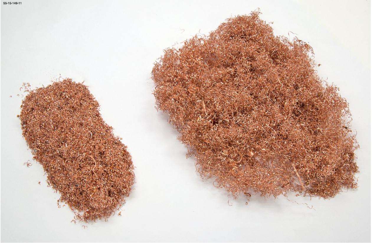
Figure 2: Bird nest turnings pictured on right and the remaining turnings on the left.
