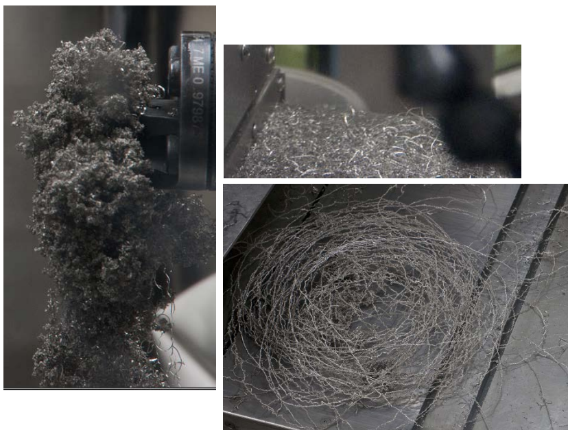
Figure 4: T-base 2 Pu turnings are hanging off the tool post (left); turnings on lathe surfaces (right).
