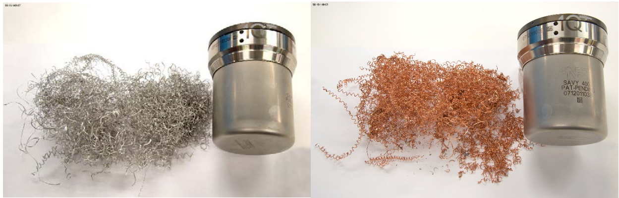
Figure 6: 500 grams of Pu equivalent volume next to one quart Savy container.
