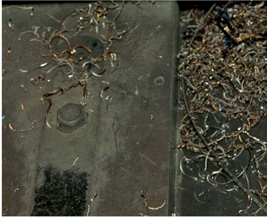
Figure 5: Pu turnings produced on the waist band lathe.
