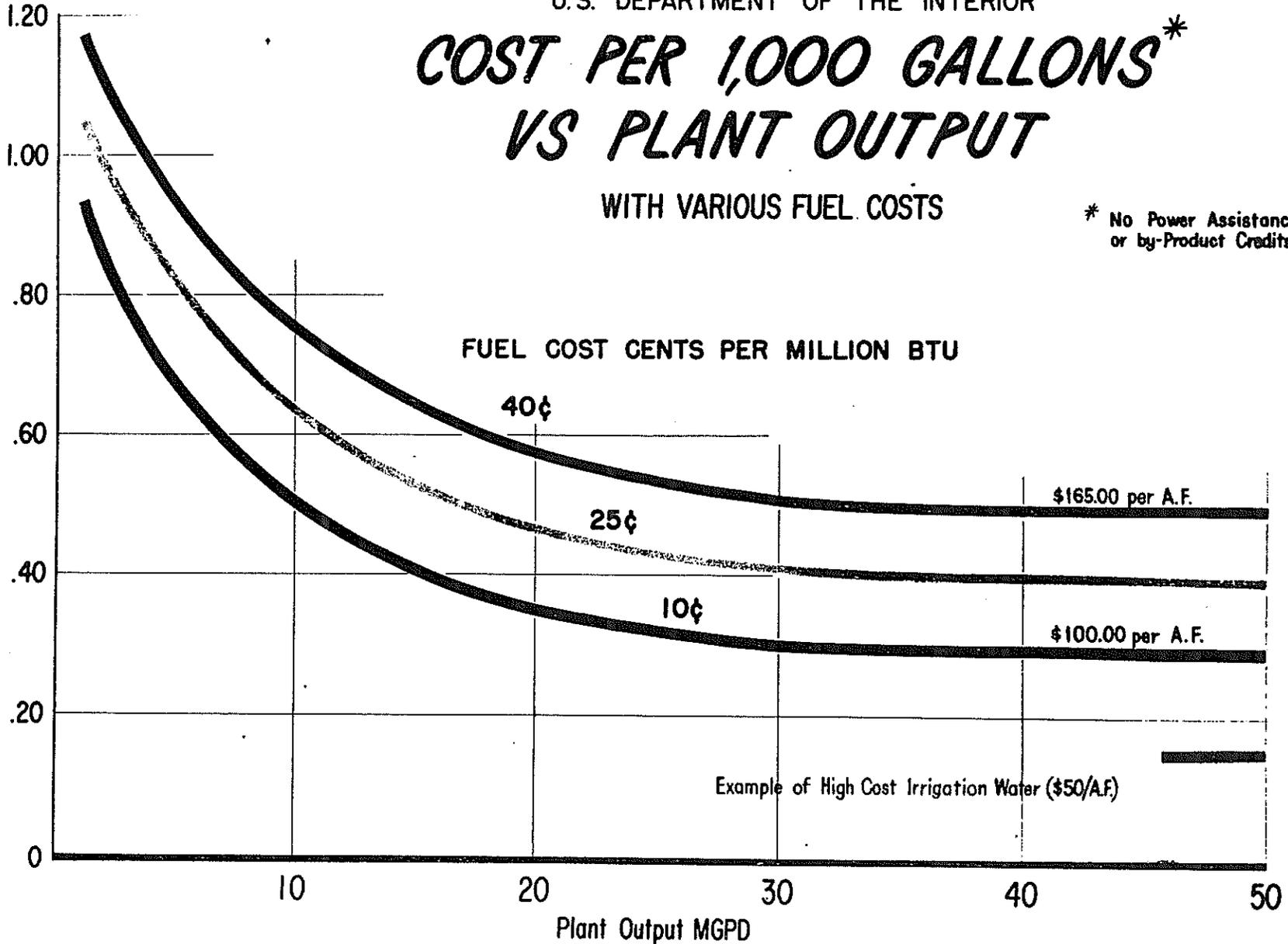
represents the cost of water per thousand gallons. The horizontal ordinate represents the plant output in million gallons per day. The Department's largest sea water conversion plants, the one in Freeport, Texas, and also the one at San Diego, California, both have a capacity of 1,000,000 gallons per day. Their costs are about \$1.00 to \$1.25 per 1,000 gallons. You can see the economies we anticipate as we construct larger plants utilizing presently known processes.
