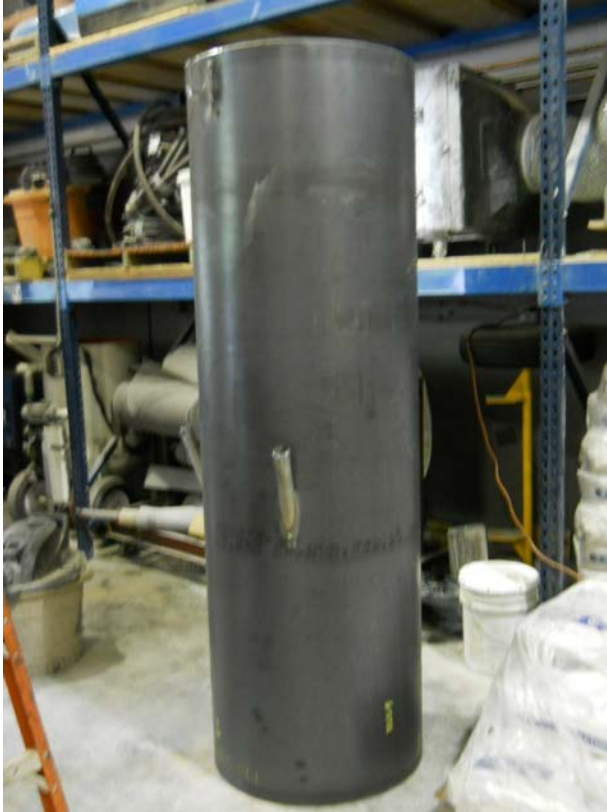
Reducer and Dipleg Sections Before Refractory Installation
