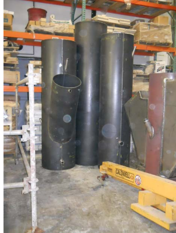
Reducer and Dipleg Sections Before Refractory Installation
