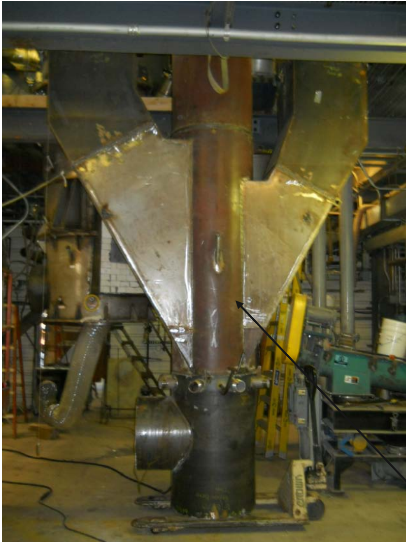
'Cactus' with Fluidizing Section and Seal Pot Connections Assembled on Ground Level
