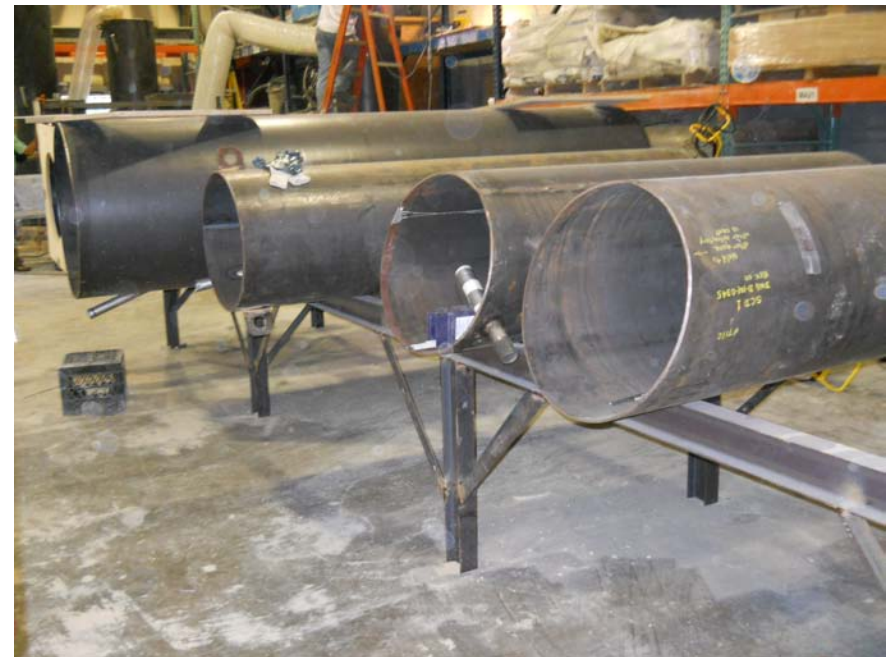
Reducer and Dipleg Sections Lined up for Refractory Installation
