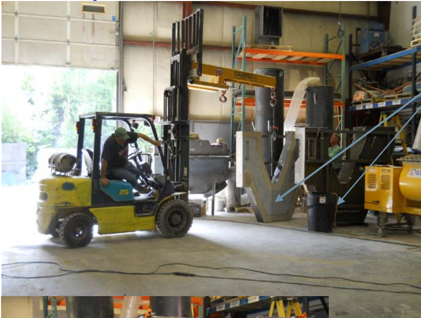
Reducer to Oxidizer Crossover (constructed in two halves)
