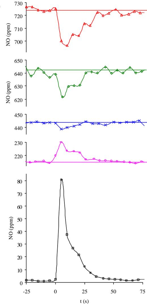
Ⓢ NO profiles after fuel injection at  $t = 0$  s
