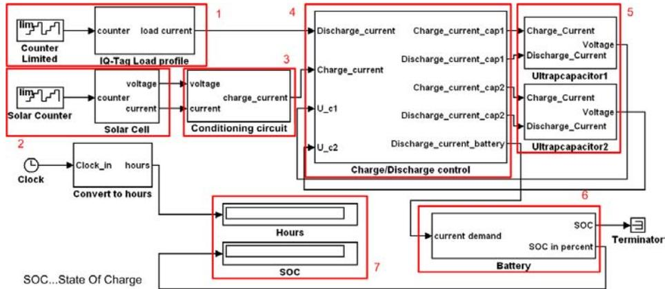
Fig. 10. Detailed structure of the simulation model
