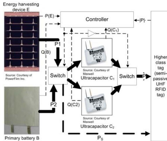
Fig. 8. Energy storage architecture variant 1 with two ultracapacitors
