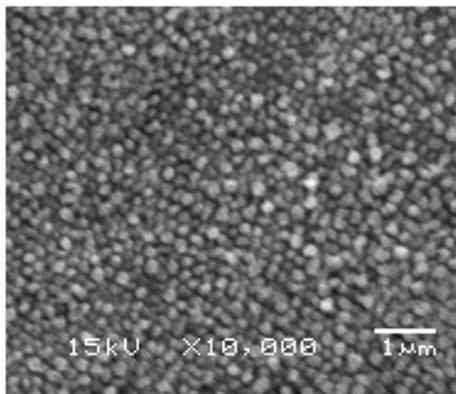
Fig. 1. SEM micrograph of ZnSe nano-dots.
