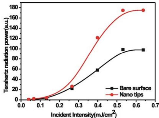
Fig. 2. THz fluence as a function of pump fluence for nano-dot and bulk ZnSe samples.
